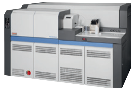
Figure 2. Thermo Scientific NEPTUNE Plus MC-ICP-MS.
