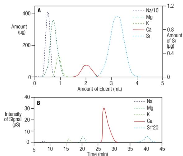
Figure 2. Elution curves for (A) classical Ca-exchange chromatography of a seawater sample (AG50W-X8, 200–400 mesh Biorad™ resin, 1.5 N  $\text{HCl}$  as eluent, recovery yield ~70%), and (B) automated high pressure ionic chromatography of a soil sample (Dionex CS16 cation-exchange column, methanesulfonic acid as eluent, recovery yield ~100%). The overall Ca blank contribution from the HPIC system was ~30 ng, i.e. ~0.5‰ of the sample Ca amount.<sup>12</sup> (Figure 2B modified after ref. 12).
