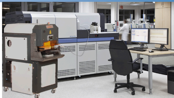
Thermo Scientific NEPTUNE Plus MC-ICPMS and Photon Machines Analyte.G2 193 nm LA system.
