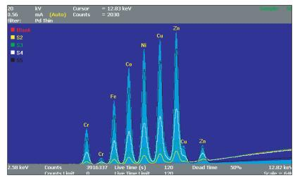
Spectra of all standards and a Blank (in red) collected under conditions optimized for Cr-Zn. The difference in background (on the right side of the spectrum) between the various samples is due to a decrease in X-ray scatter as the density of the samples increases
