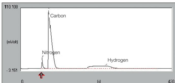
Figure 7. Typical CHN chromatogram.
