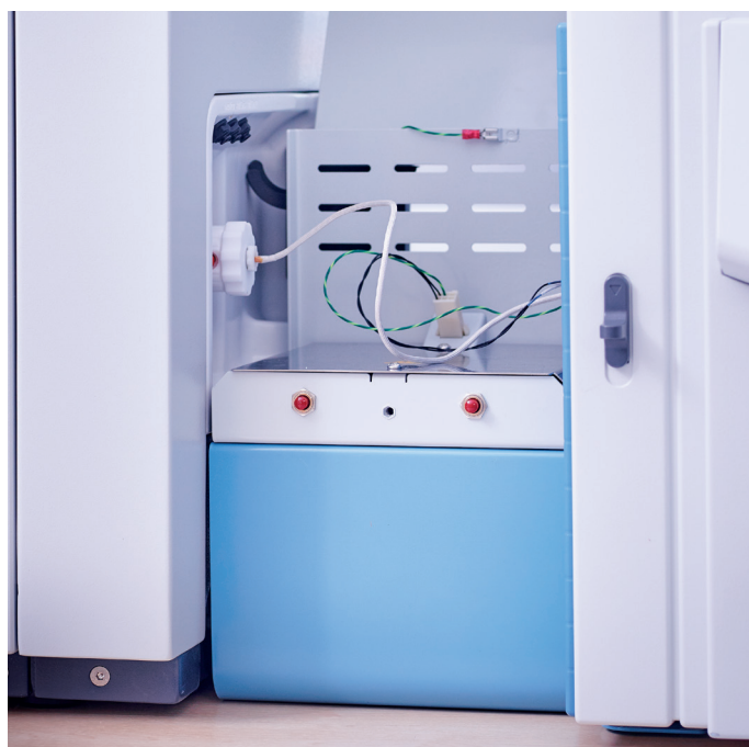
Figure 1. New GC-ICP-MS hyphenation with GCI 100 Interface.
