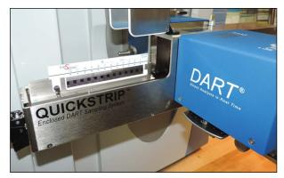
Figure 3. DART QuickStrip direct injection source.
