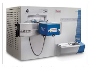
Figure 1. DART source coupled to LTQ ion trap mass spectrometer.
