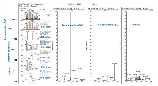
Figure 9. Data collected for acetaminophen and codeine in a pharmaceutical pill. The first column shows chronograms of TIC, full scan of targeted compound reconstructed with 5 ppm mass accuracy, and the data-dependent MS2 scans. The remaining columns show resulting MS2 spectra.
