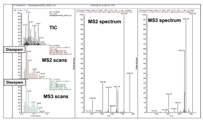
Figure 7. Data collected for diazepam in a pharmaceutical pill. The first column shows chronograms collected for the TIC, and triggered MS2 and MS3 scans for diazepam. The next two columns show representative MS2 and MS3 spectra collected for diazepam.
