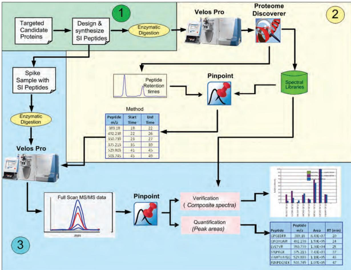
Figure 2. Optimized workflow: 1) Design, synthesis and preparation of stock solutions of SI peptides; 2) Optimization of chromatography and creation of an inclusion list for a scheduled full-scan MS/MS method; 3) Run scheduled full-scan MS/MS to create standard curves and evaluate unknown samples.
