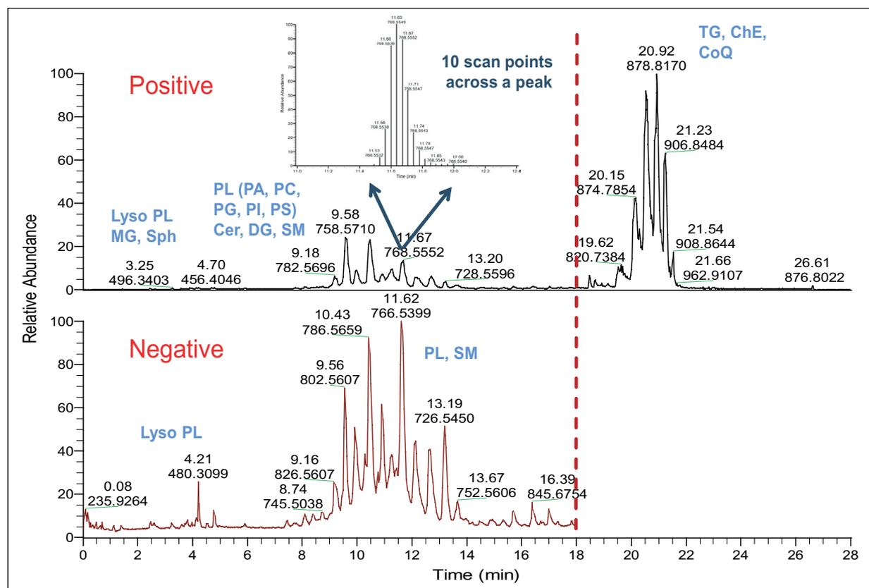
Figure 7. Base peak chromatograms of positive and negative ion modes of bovine heart lipid extracts in a single run using the novel intelligent comprehensive workflow.
