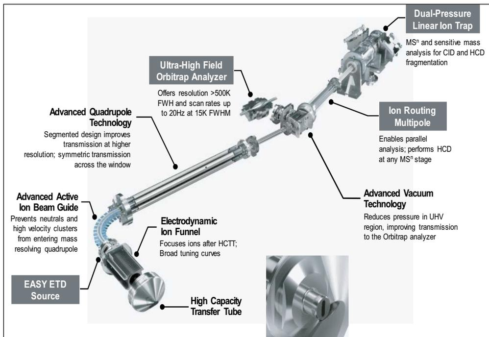
Figure 1. Instrument layout of Orbitrap Fusion Lumos Tribrid mass spectrometer.
