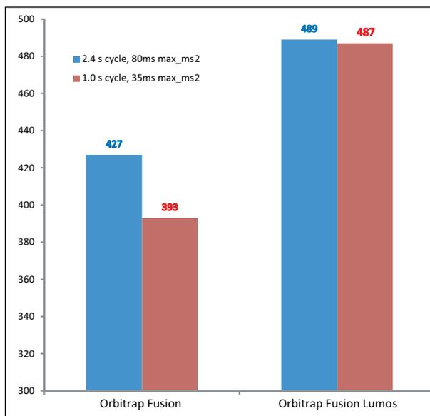
Figure 3. Comparison of Lipid IDs in 1  $\mu\text{g}$  of bovine heart lipid extract with the Orbitrap Fusion MS and Orbitrap Fusion Lumos MS Instruments with 1.0 second and 2.4 second cycle times. The number of lipid IDs were determined using an average of duplicate positive data dependent HCD MS<sup>2</sup> runs.
