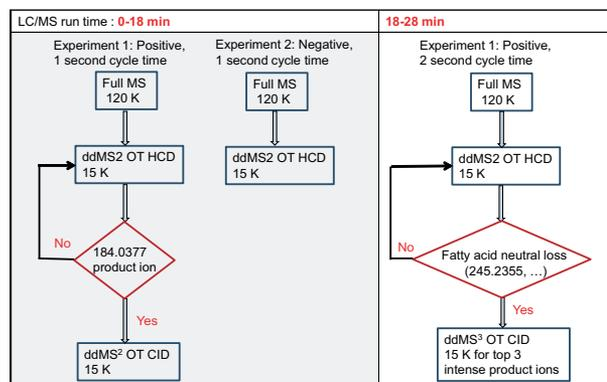
Figure 2. Flow chart of comprehensive HCD MS<sup>2</sup> and CID MS<sup>2</sup>/MS<sup>3</sup> workflow.
