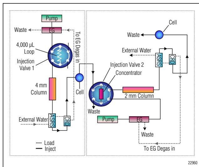
Figure 1. Schematic diagram of two-dimensional system for the determination of trace concentrations of perchlorate.
