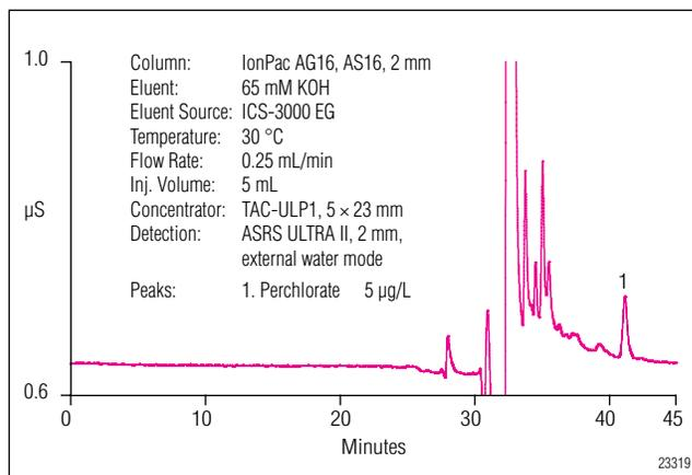
Figure 3. Chromatogram of a 0.5 µg/L perchlorate standard with the IonPac AS16 column in the second dimension.
