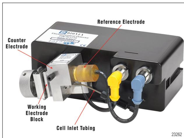
Figure 1. Amperometry cell.
