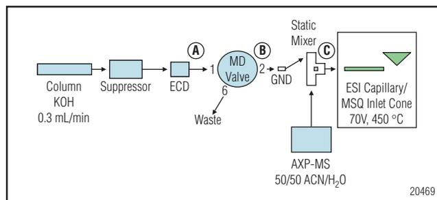
Figure 1. Flow diagram showing IC-MS with matrix diversion.
