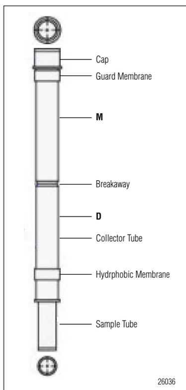
Figure 1. MICRO DIST tube assembly<sup>14</sup>
