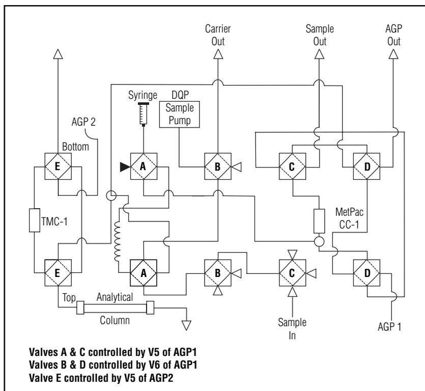
Figure 2. Schematic of chelation ion chromatography system.
