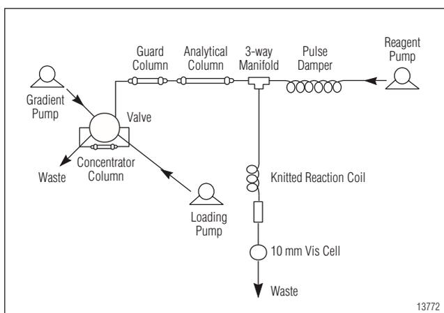
Figure 1 System configuration for detection of transition metals
