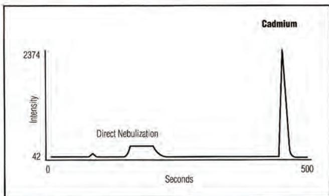
Figure 1 A typical scan of trace metal analysis by IC/ICAP
