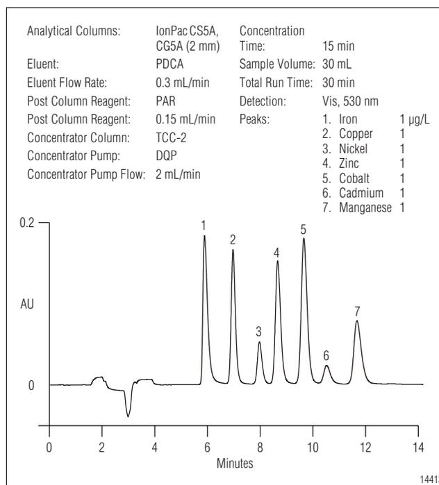
Figure 2 1 µg/L (ppb) transition metals standard (30 mL concentrated)
