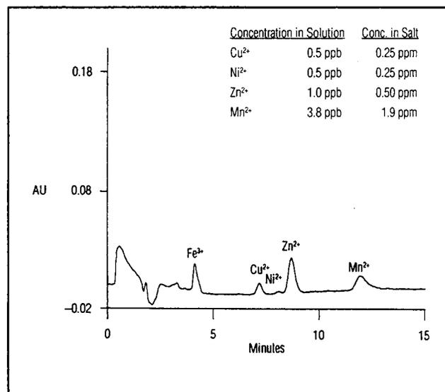
**Figure 1** Transition metals in reagent grade magnesium chloride
