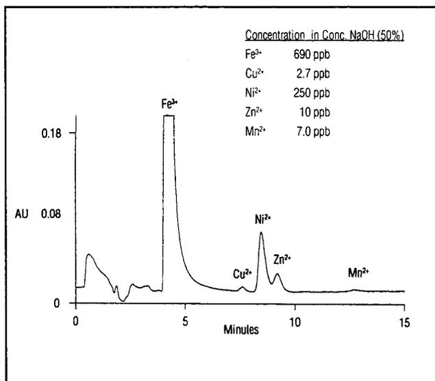
Figure 2 Transition metals in sodium hydroxide
