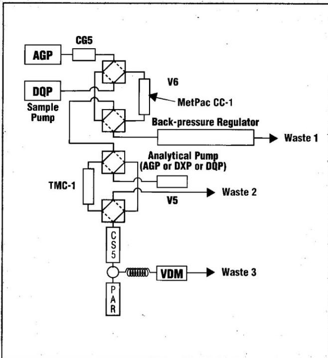
Figure 3 Schematic of Chelation IC System 1
