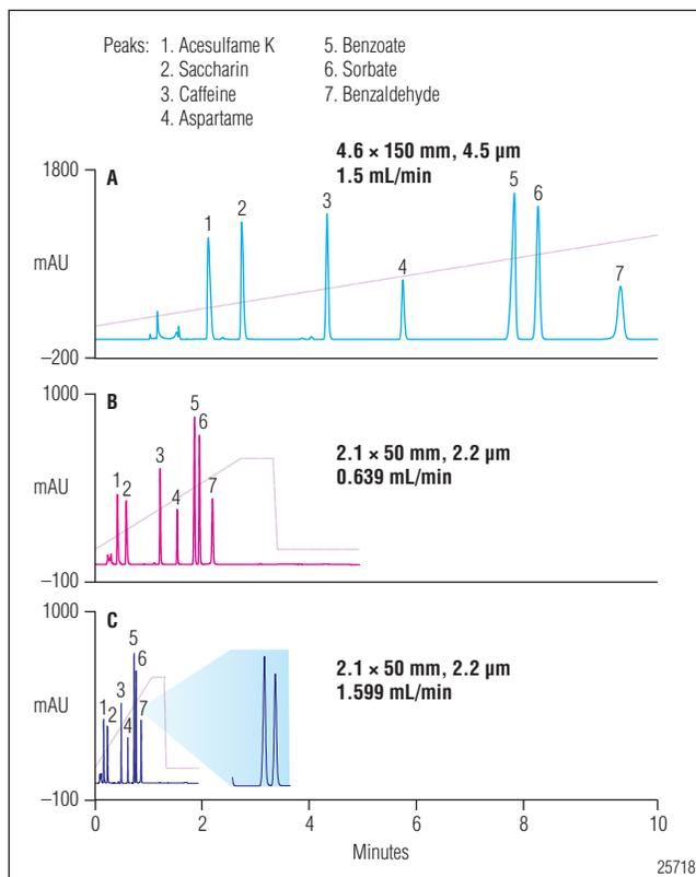
Figure 4. Method transfer with the Method Speed-Up Calculator from A) a conventional LC separation on an Acclaim 5  $\mu$ m particle column, to B) and C) RSLC separations on an Acclaim 2.2  $\mu$ m particle column.
