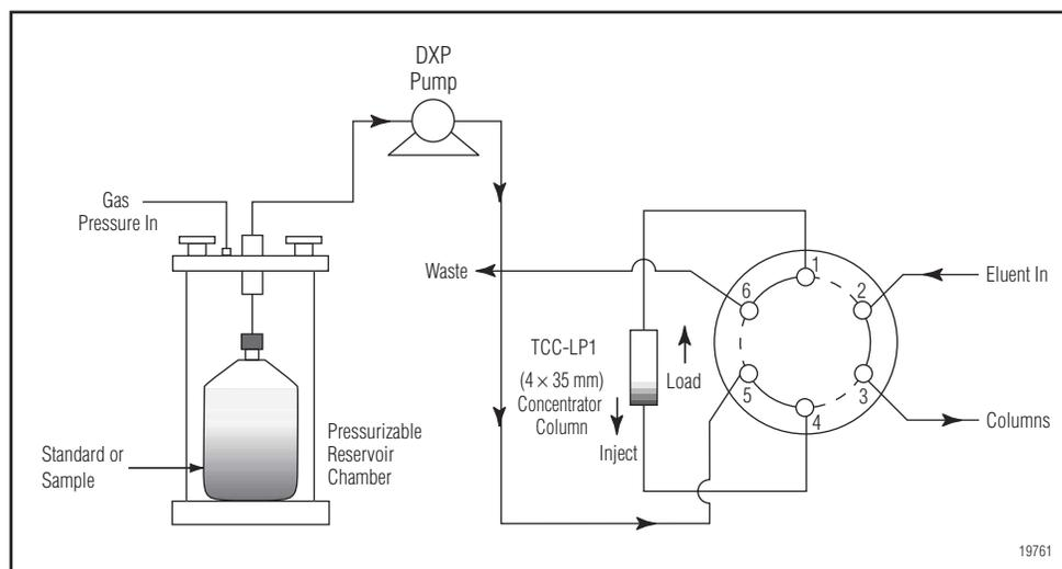
Figure 1. Ion chromatography preconcentration system (sample loading position shown).
