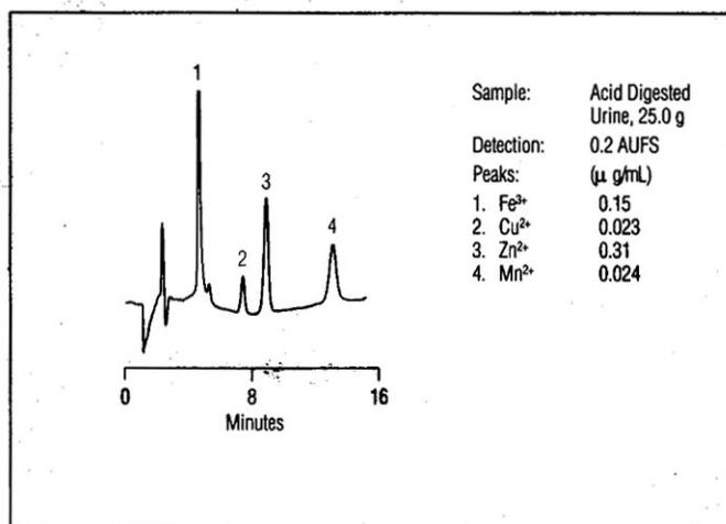
Figure 12 Determination of transition metals in urine using Chelation IC
