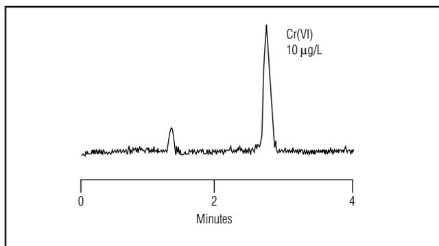
Figure 2. Determination of Cr(VI) in water, waste water, and solid waste extracts.
