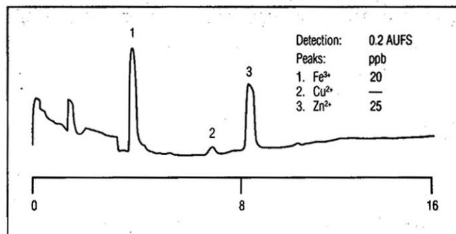
Figure 8 Typical blank obtained using Chelation Ion Chromatography
