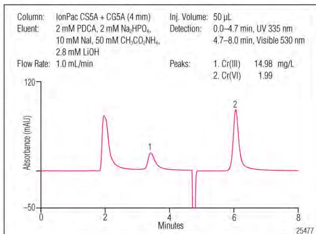
Figure 3. Chromatogram of a 15 mg/L Cr(III) standard.
