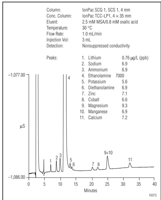
Figure 6. Chromatogram of a simulated feed water sample.
