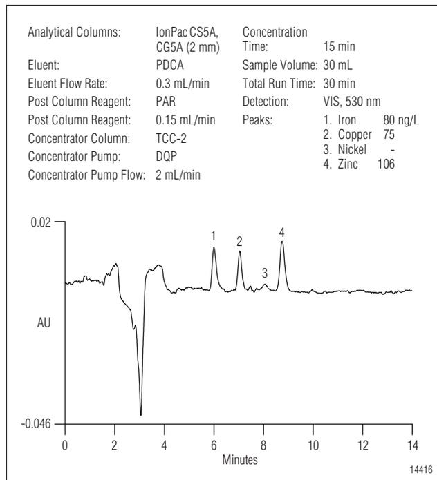
**Figure 5** SC2 batch (30 mL concentrated) containing 1 mL HCl / 5 mL H<sub>2</sub>O<sub>2</sub> / 494 mL H<sub>2</sub>O
