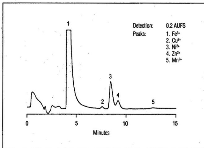
Figure 10 Determination of transition metals in sodium hydroxide using Chelation IC
