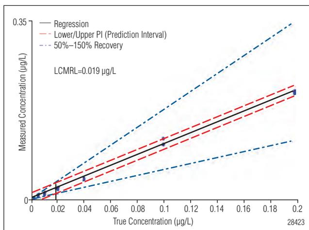
Figure 4. Determination of the LCMRL using LCMRL calculator.
