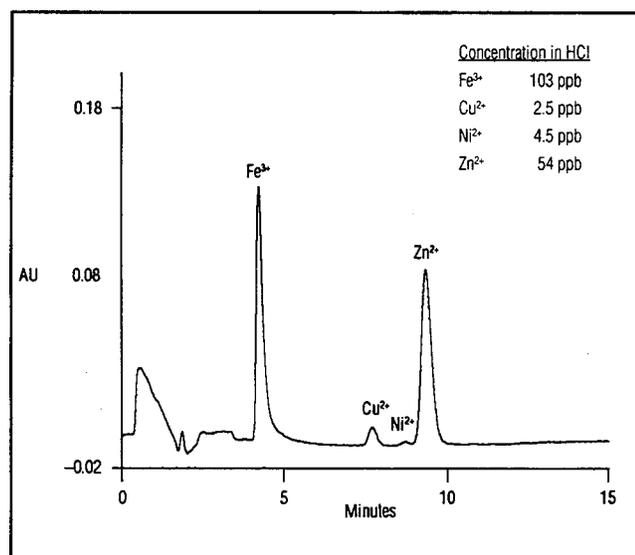
Figure 3 Trace metals in hydrochloric acid
