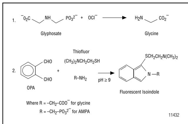
**Figure 6** Postcolumn reaction chemistry of glyphosate and AMPA.
