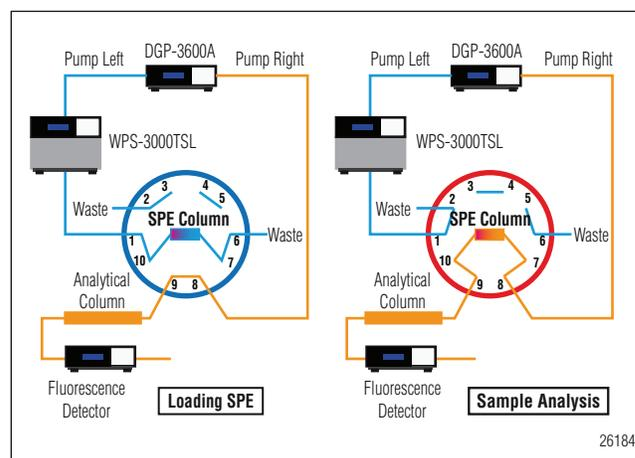
Figure 3. Schematic of devices for determination of LAS using on-line SPE followed by HPLC with fluorescence detection.
