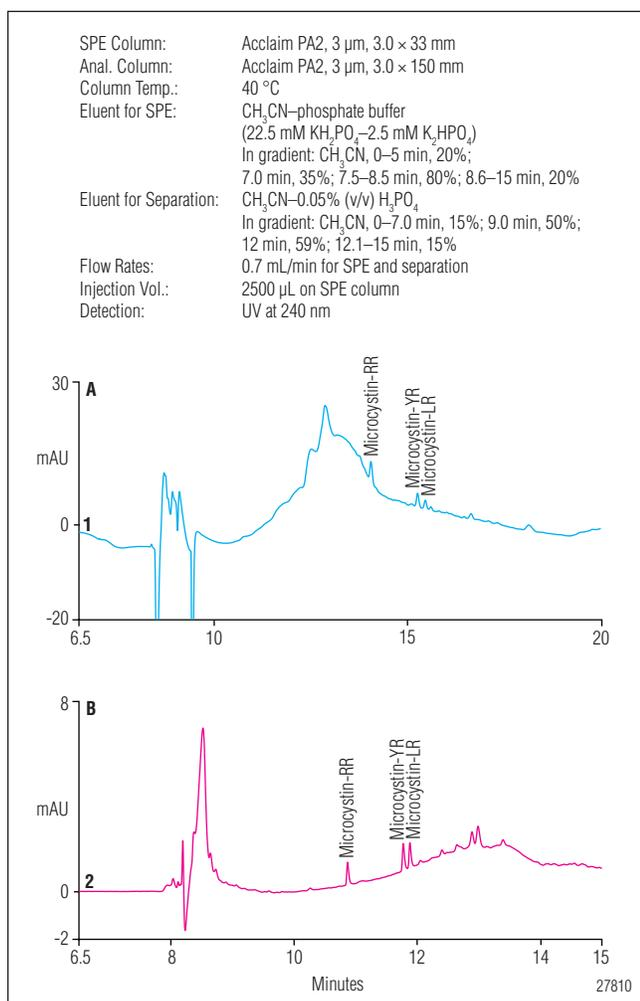
Figure 5. Chromatograms of a tap water sample spiked with 0.5  $\mu$ g/L each of microcystin-RR, -YR, and -LR standard using different target-cut modes. A) Valve-switching starts from microcystin-RR and ends at microcystin-LR when they are eluted from the SPE column. B) The three microcystins elute together from the SPE column.
