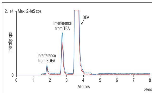
Figure 3. Chromatographically separated MRM interferences for DEA.
