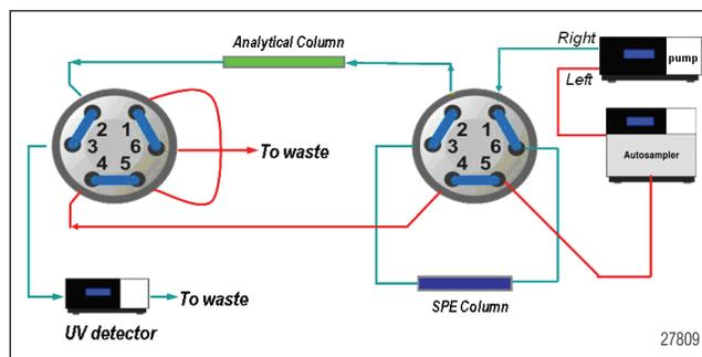
Figure 4. Flow schematic for the target-cut on-line SPE method equipped with two 2p-6p valves.
