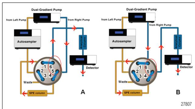
Figure 2. Flow schematics for A) traditional and B) target-cut on-line SPE methods equipped with one 2p–6p valve for sample preparation and analysis.
