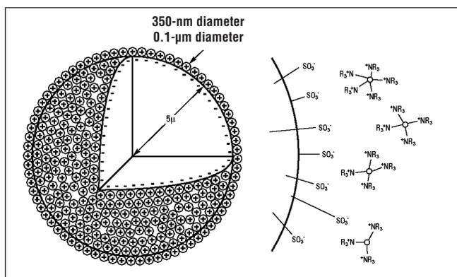
Figure 1. Pellicular anion-exchange resin bead.
