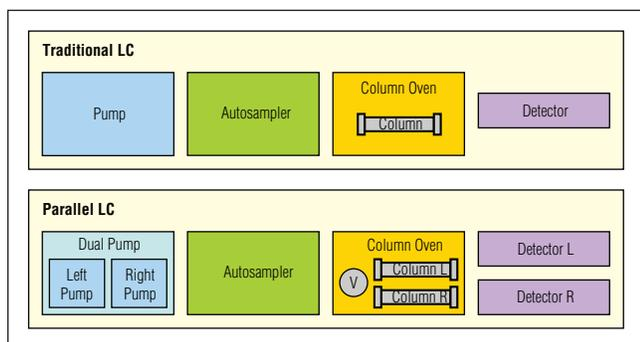
Figure 1. Schematic instrument setup for traditional and Parallel LC. Compared to a traditional setup, Parallel LC nearly doubles throughput by only adding a pump, a detector, and a switching valve (V). The autosampler and the column oven are shared between the two separation channels (sub-systems).
