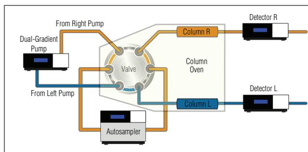
Figure 2. Flow scheme for UltiMate 3000 Parallel LC mode. The autosampler is currently in the flow path of the right pump. (A Dionex UltiMate DGP-3600 ×2 Dual-Gradient Pump encloses two ternary low-pressure gradient pumps in a single housing. The sub-devices are called left pump and right pump.)
