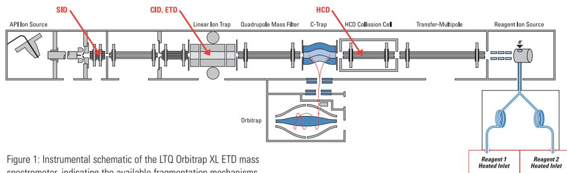
Figure 1: Instrumental schematic of the LTQ Orbitrap XL ETD mass spectrometer, indicating the available fragmentation mechanisms
