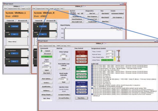
Figure 9. Panel Tabsets provide well structured overview and easy control possibilities for the two sub-systems. The screen can be shared between the sub-systems (as in the background) or it can be filled with the controls of a single module (as in the foreground).
