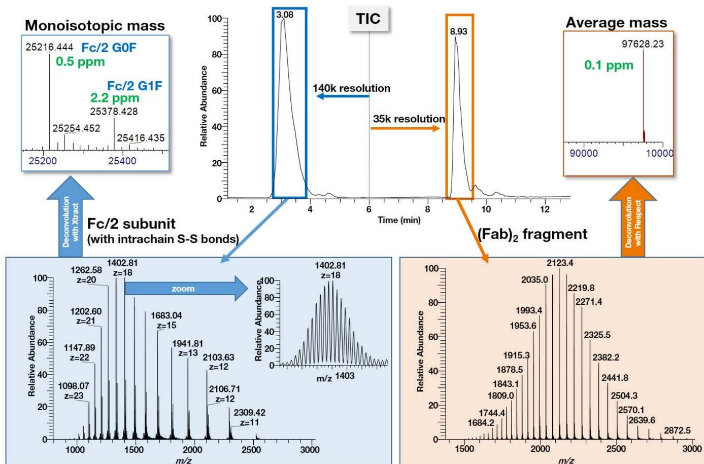
Figure 9. Total ion chromatogram and obtained MS spectra of trastuzumab after FabRICATOR digest without reduction resulting in the Fc/2 and (Fab')<sub>2</sub> regions with both subunits bearing intact disulfide bonds, resulting in observed molecular weights of ~25 kDa for the Fc/2 subunits and ~97 kDa for the (Fab')<sub>2</sub> fragment.
