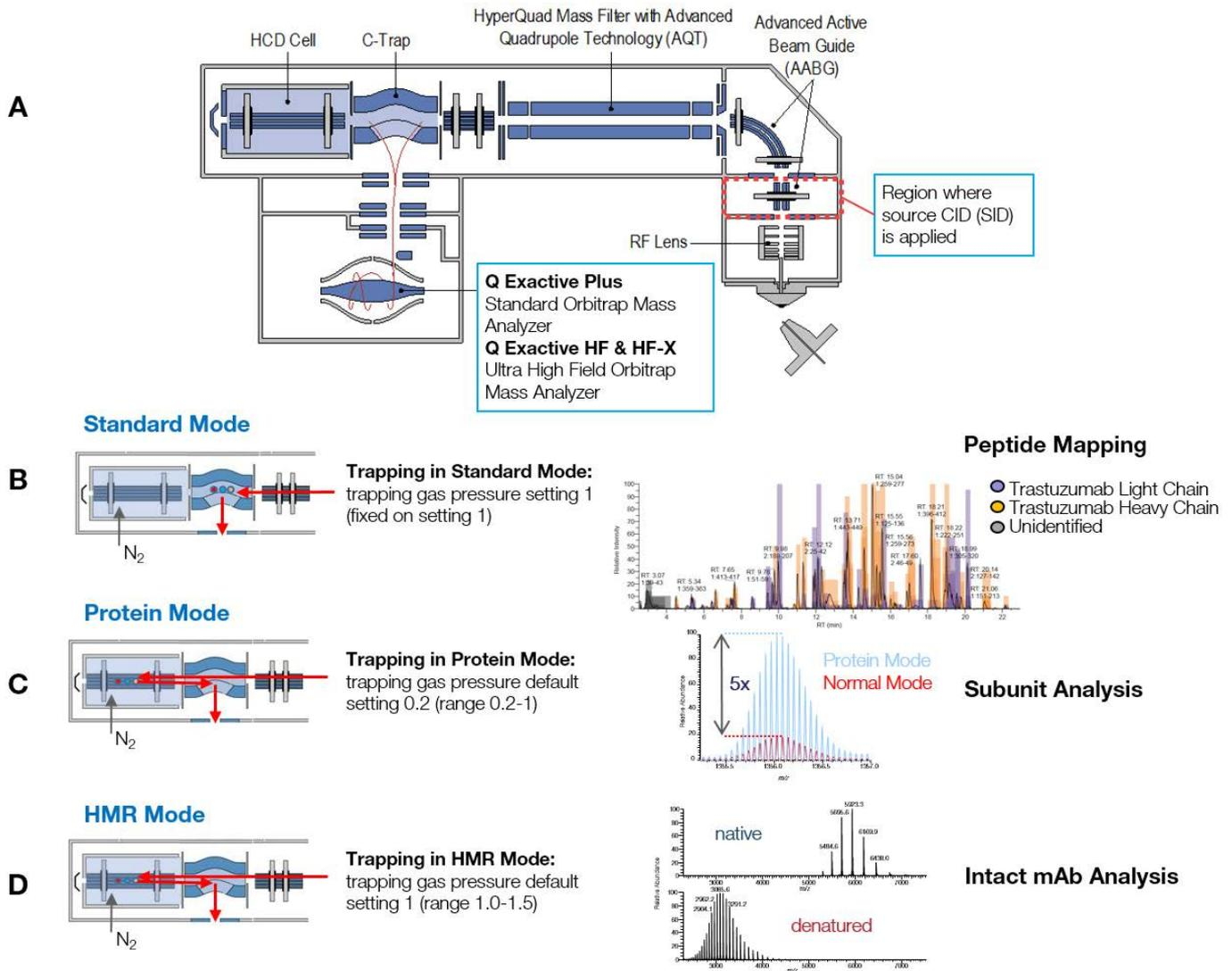
Figure 3. A) Schematic of the Q Exactive Plus and Q Exactive HF mass spectrometers and differences in the trapping path in the three different operating modes available: B) Standard Mode, C) Protein Mode and D) HMR Mode.
