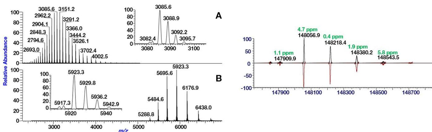
Figure 4. Full MS spectra acquired from intact trastuzumab under denaturing (A) and native conditions (B).
