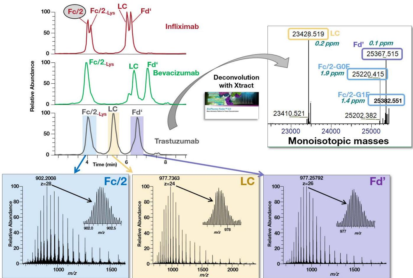
**Figure 10.** Total ion chromatograms of separated subunits obtained after FabRICATOR digest and reduction from trastuzumab, bevacizumab, and infliximab. Obtained Full MS mass spectra and baseline-resolved isotope patterns of the individual charge states, as well as the result after deconvolution, is showcased for trastuzumab.
