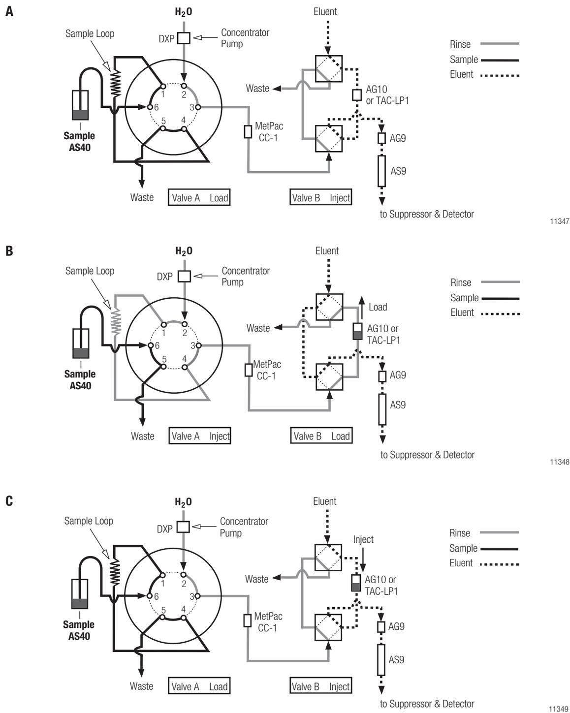
Figure 4. Preconcentration suppressed IC system configuration. (A) sample loaded into loop; (B) sample washed onto concentrator column; (C) retained anions eluted to Dionex IonPac AG9/AS9-SC analytical column set.
