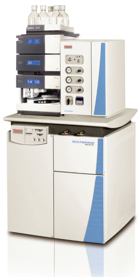
Figure 1. The Thermo Scientific LC-IRMS system.
