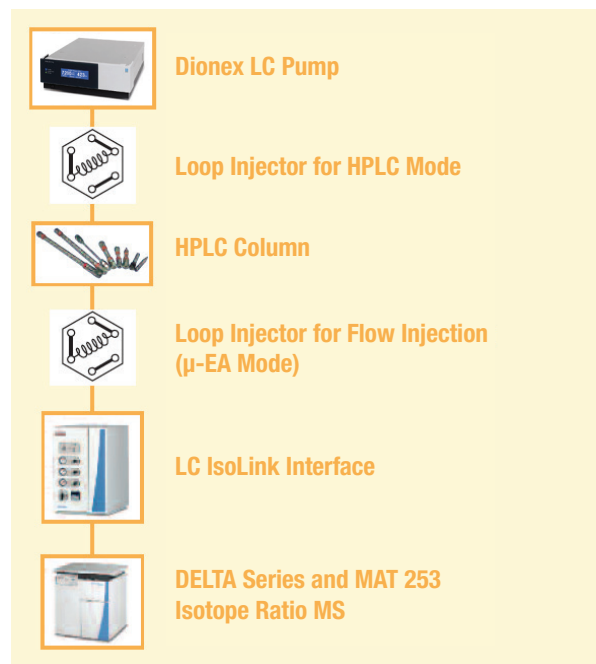
Figure 3. Scheme of the Thermo Scientific LC-IRMS workflow with the LC IsoLink LC-IRMS.
