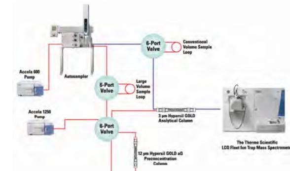
FIGURE 2A. LCQ Fleet Mass Spectrometer Method. Dedicated MS/MS Using Mass List. Simplified method, only uses one segment.
