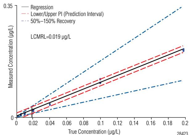
Figure 4. Determination of the LCMRL using LCMRL calculator.
