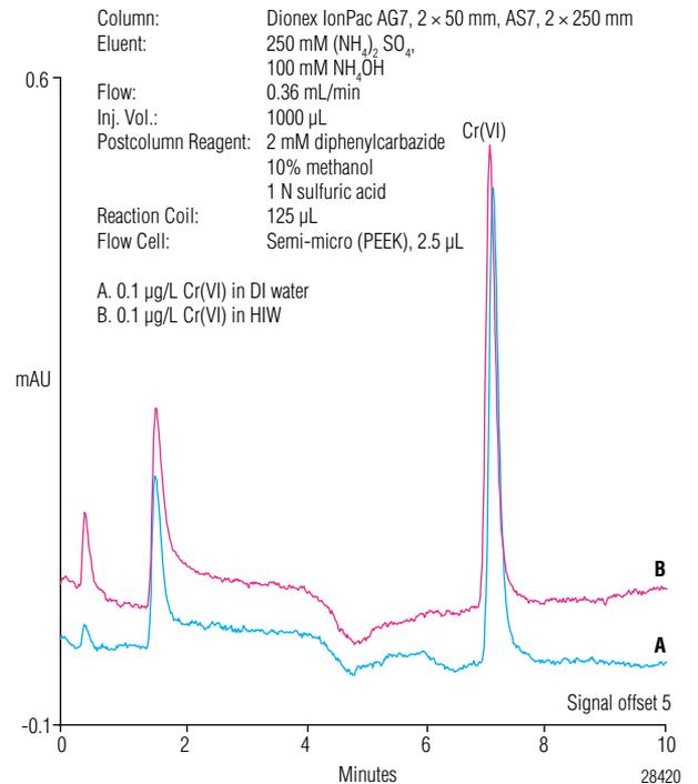
Figure 1. Determination of Cr(VI) (0.1 µg/L) in A) DI water and B) HIW on a Dionex ICS-3000 system. Postcolumn reagent delivered by a DP pump. Flow cell: semi-micro (PEEK).
