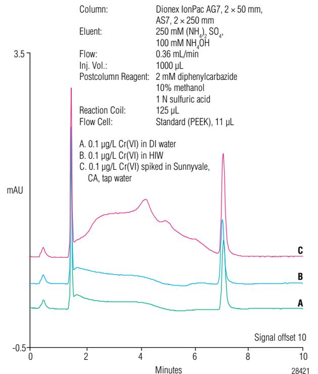
Figure 2. Determination of Cr(VI) in A) DI water, B) HIW, and C) Sunnyvale, CA, tap water using a Dionex ICS-3000 system. Sunnyvale, CA, tap water blank has a background Cr(VI) level of 0.05 µg/L Cr(VI). Postcolumn reagent delivered by an AXP pump. Flow cell: standard (PEEK).
