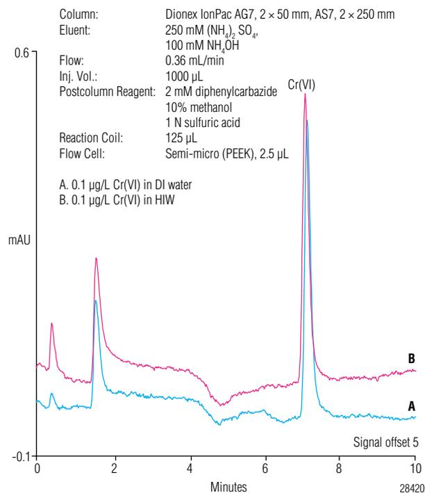
Figure 1. Determination of Cr(VI) (0.1 µg/L) in A) DI water and B) HIW on a Dionex ICS-3000 system. Postcolumn reagent delivered by a DP pump. Flow cell: semi-micro (PEEK).
