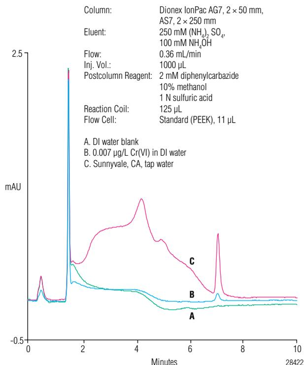
Figure 3. Determination of Cr(VI) in A) DI water blank, B) 0.007  $\mu\text{g/L}$ , and C) Sunnyvale, CA, tap water blank on a Dionex ICS-3000 system. Postcolumn reagent delivered by the second pump of DP. Flow cell: standard (PEEK).
