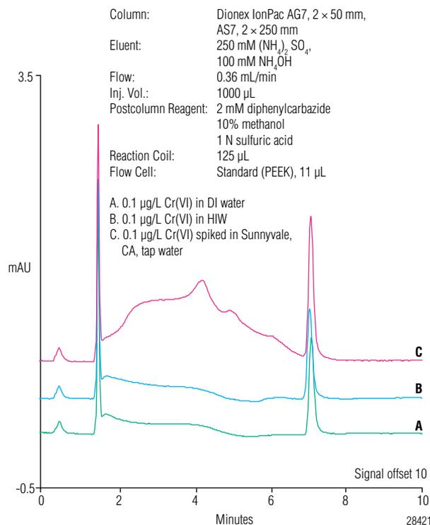
Figure 2. Determination of Cr(VI) in A) DI water, B) HIW, and C) Sunnyvale, CA, tap water using a Dionex ICS-3000 system. Sunnyvale, CA, tap water blank has a background Cr(VI) level of 0.05 µg/L Cr(VI). Postcolumn reagent delivered by an AXP pump. Flow cell: standard (PEEK).
