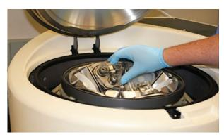
Figure 4. Dionex ASE Pucks are loaded into the Rocket Evaporator.
