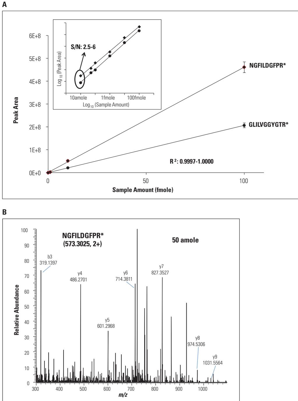
Figure 5. Amounts of heavy peptide standards and measured peak area in SIM scan were plotted and analyzed by linear regression fitting with 1  $\mu\text{g}$  of yeast tryptic digest as background. A) Linear regression fittings and standard deviations for two heavy peptide standards. The  $R^2$  of linear fitting is shown to be above 0.9991. The insert shows linear fitting of the same data in  $\log_{10}$  space. B) HCD spectrum for NGFILDGFPR\* ( $m/z$  573.3025, 2+) with major y ions labeled.
