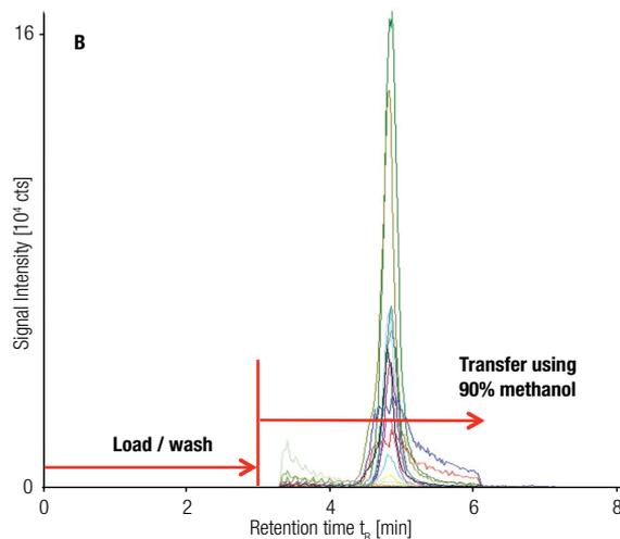
Figure 5. Backflush on-line SPE trapping and elution of polar (A) and non-polar coccidiostats (B) on SolEx HRP cartridges (no analytical column connected).
