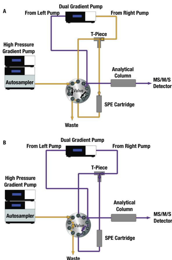
Figure 2. Flow schemes of the advanced on-line SPE configuration for loading/washing (A) and transfer/analysis (B).
