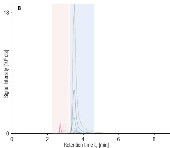
Figure 4. Foreflush on-line SPE trapping and elution of coccidiostats on Cyclone-P (A) and SolEx HRP (B) cartridges.
