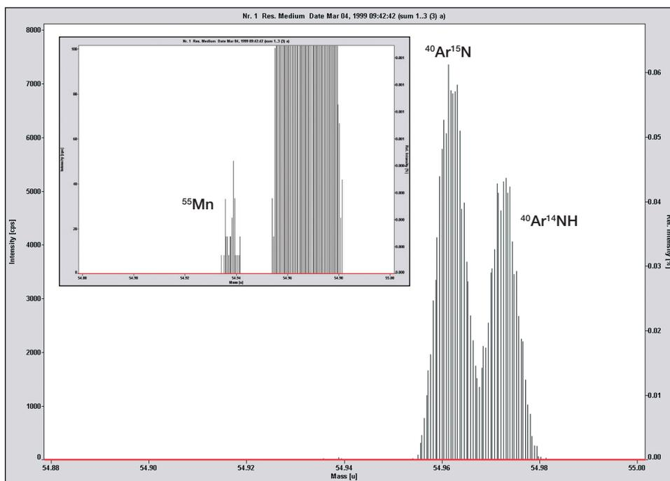
Figure 2. Medium resolution ( $R = 4000$ ) spectrum of manganese ( $m/z$  55) showing  $^{40}\text{Ar}^{15}\text{N}$  and  $^{40}\text{Ar}^{14}\text{NH}$  interferences generated by the TMAH matrix.
