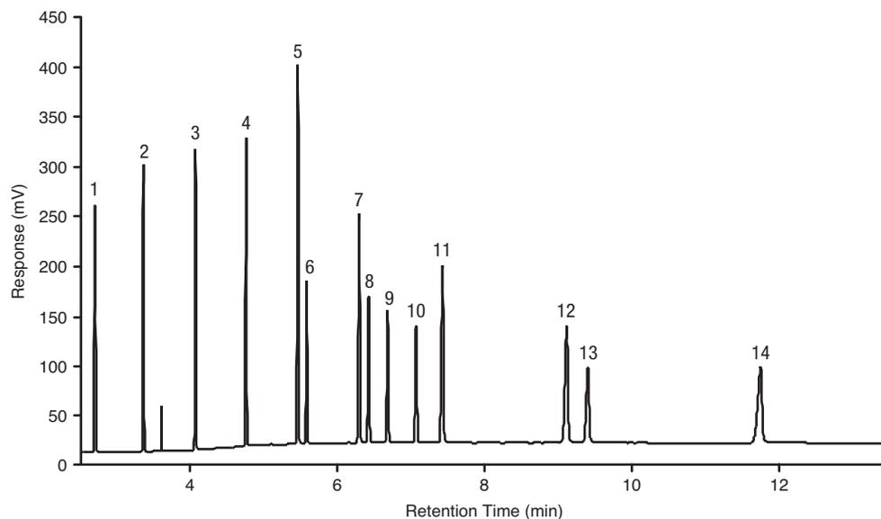
Figure 2: 1% C8–C24 FAMES solution separated on a TraceGOLD TG-WaxMS fused silica GC column
