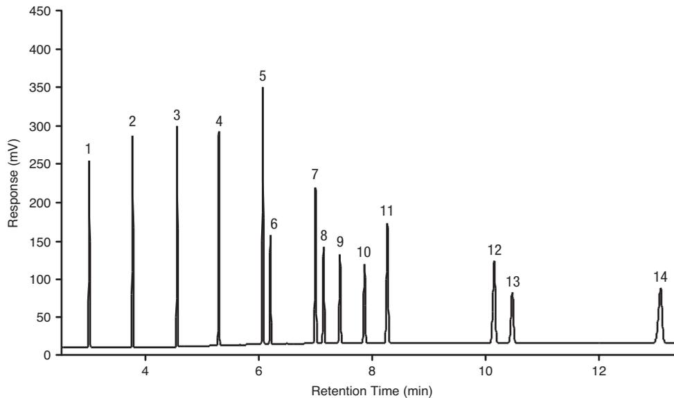
Figure 1: 1% C8–C24 FAMES solution separated on a TraceGOLD TG-WAXMT metal GC column
