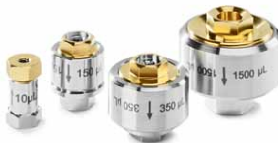
Figure 13. The range of static mixers within the Dionex UltiMate 3000 SpinFlow product line.
