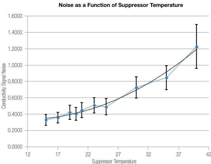
Figure 2. CD cell temperature was kept constant at 47 °C. Error bars show a single standard deviation of recorded noise values over a period of one hour.
