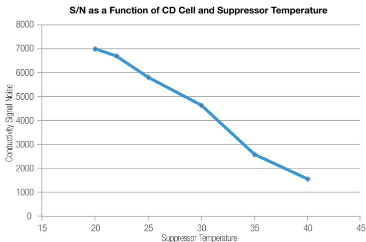
Figure 4. CD cell temperature was varied with a constant +7  $^{\circ}$ C difference to the suppressor temperature. To determine signal strength, a 15  $\mu$ L injection of 10 ppm sulfate standard was injected.
