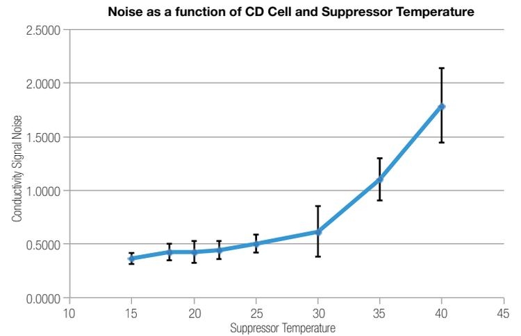
Figure 3. CD cell temperature was varied with a constant +7 °C difference to the suppressor temperature. Error bars show a single standard deviation of recorded noise values over a period of one hour.
