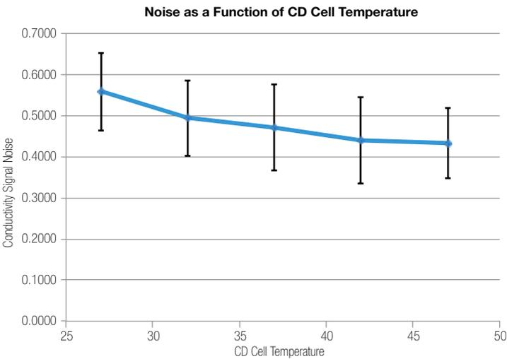
Figure 1. Suppressor temperature was kept constant at 20 °C. Error bars show a single standard deviation of recorded noise values over a period of one hour.
