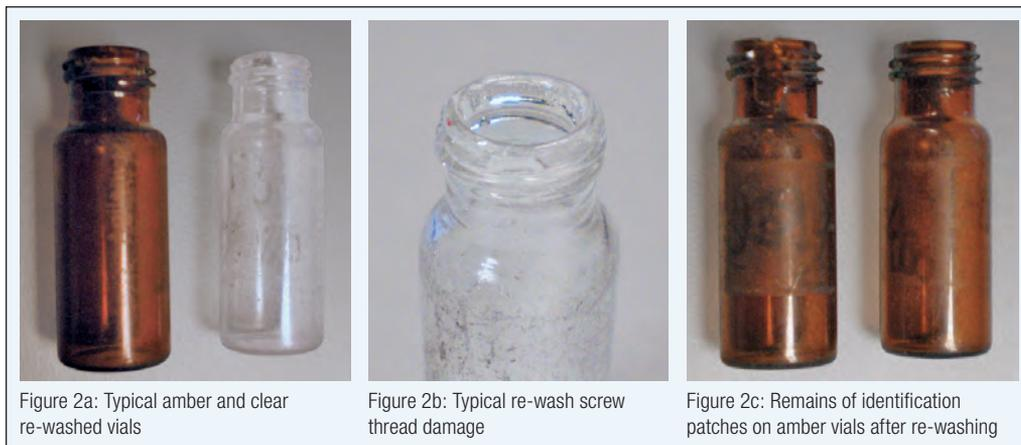
Figure 2a: Typical amber and clear re-washed vials
