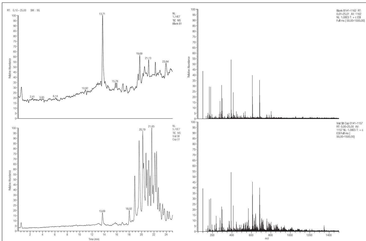
Figure 8: Comparison of blank with contaminated vial using the Silicone/PTFE septa
