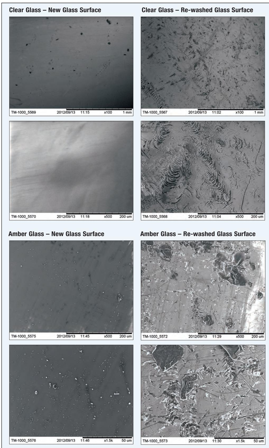
Figure 3: Comparison of new and re-washed glass vial surfaces
