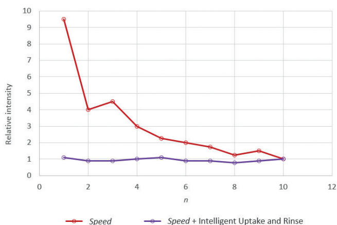
Figure 7. Relative intensities of P 177.495 nm (axial) in replicate analyses of one blank sample, after running 15 samples with P levels at 3 orders of magnitude without and with Intelligent Uptake and Rinse. n is the number of blank replicate analyses after running a highly concentrated P-containing sample.
