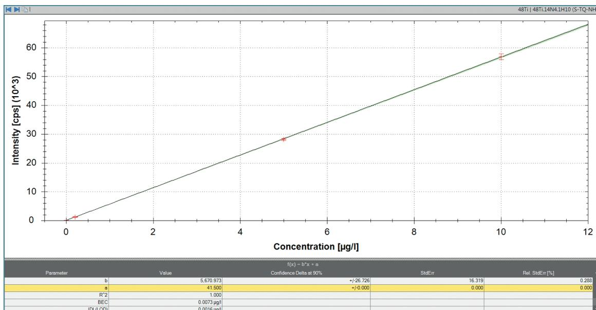
Figure 4. Calibration curve of <sup>114</sup>(Ti(NH<sub>3</sub>)<sub>3</sub>NH)\* in 1% m/m H<sub>2</sub>SO<sub>4</sub> with TQ-NH<sub>3</sub> mode.
