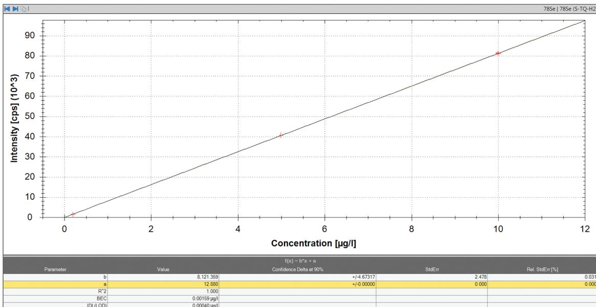
Figure 5. Calibration curve of <sup>78</sup>Se in 2% HNO<sub>3</sub> with TQ-H<sub>2</sub> mode.
