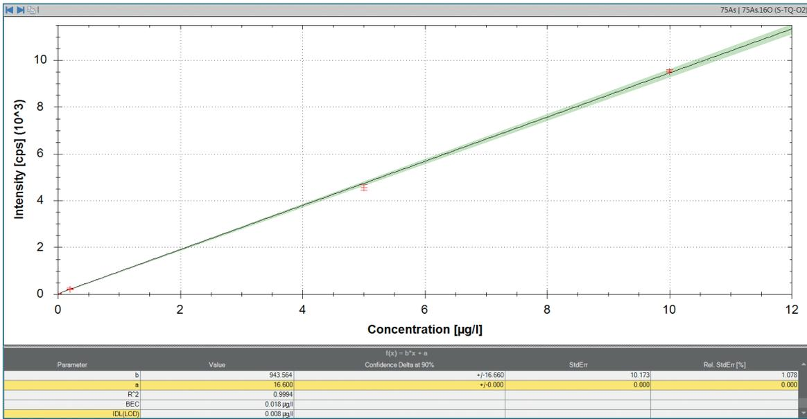
Figure 2. Calibration curve of  $^{75}\text{As}^{16}\text{O}^+$  in  $10 \text{ mg}\cdot\text{L}^{-1}$  Co with TQ- $\text{O}_2$  mode.
