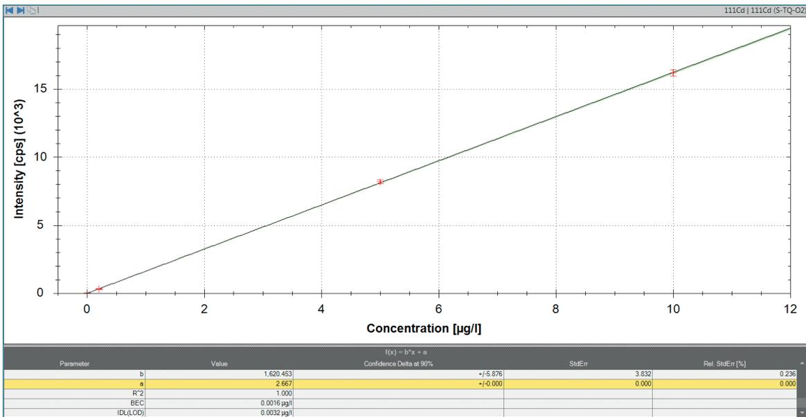
Figure 3. Calibration curve of  $^{111}\text{Cd}^+$  in  $10 \text{ mg}\cdot\text{L}^{-1}$  Mo with TQ- $\text{O}_2$  mode.
