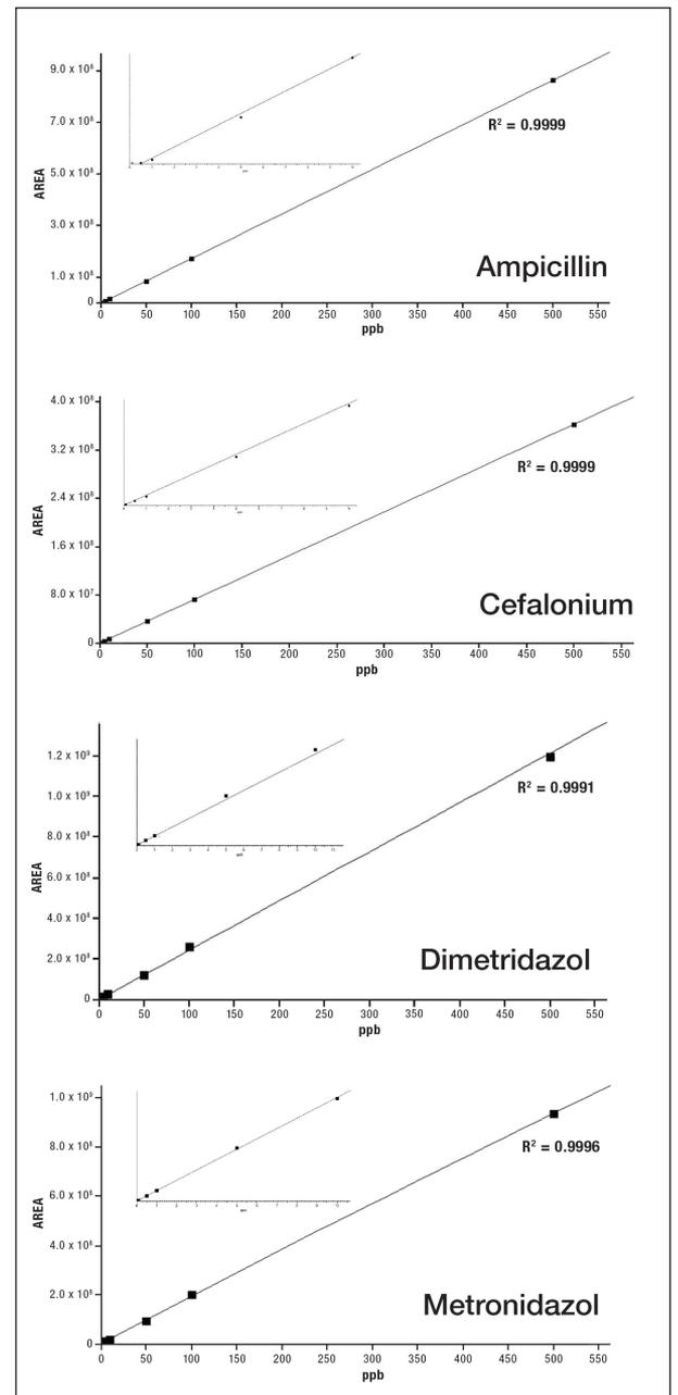
Figure 3. Selected examples of linearity for different compounds in the calibration range of 0.01–500 µg/kg.
