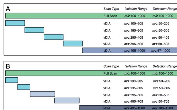
Figure 1. Examples for vDIA setup with five fragment scan windows, covering a mass range from  $m/z$  100 to 1000 (A) and from  $m/z$  100 to 1500 (B).
