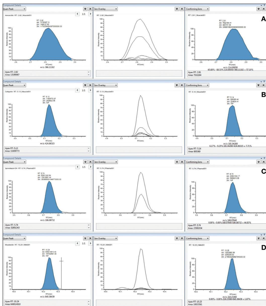
Figure 2. Selectivity of selected component in matrix; A: ampicillin in pig muscle at 5 µg/kg; B: sulfadiazin in pig kidney at 5 µg/kg; C: ronidazol in pig plasma at 1 µg/kg; D: moxidectin in cow milk at 1 µg/kg.
