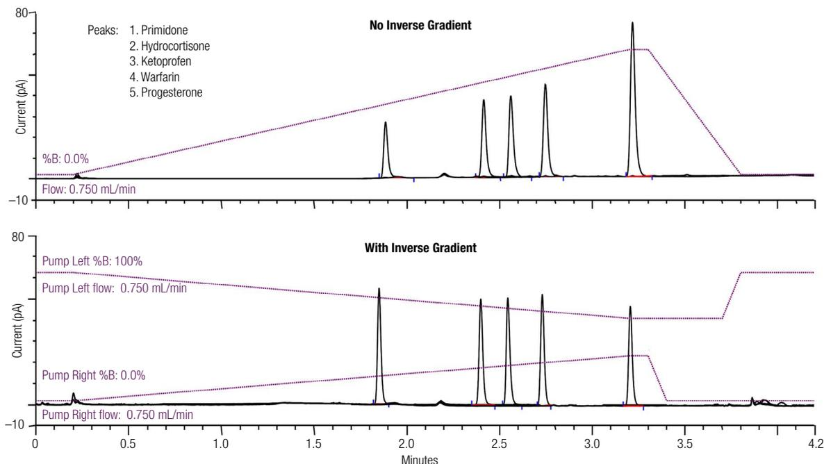
**Figure 3. Chromatograms of five pharmaceutical compounds with and without the application of an inverse gradient and charged aerosol detection.**
