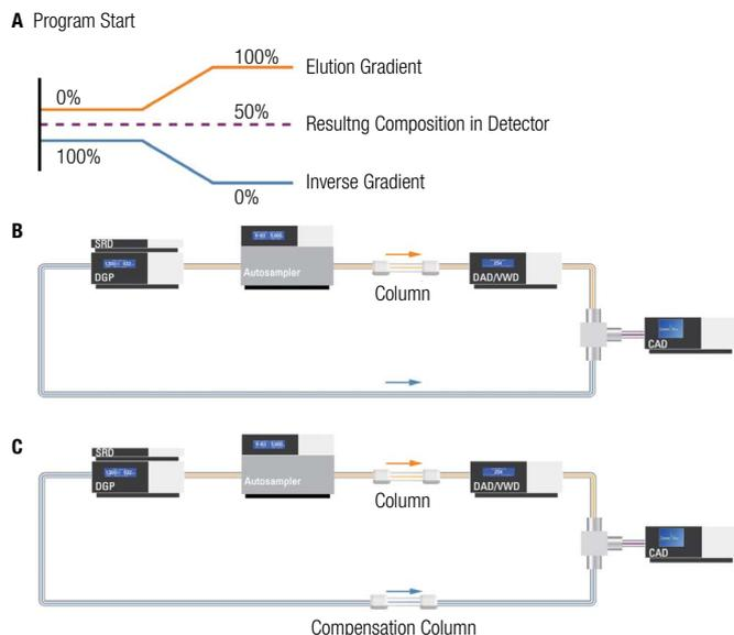
**Figure 2. Configuration of the inverse gradient with (A) giving the effect of the inverse gradient on the final solvent composition, (B) the inverse gradient setup without an additional and (C) with an additional column.**
