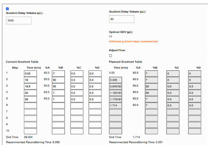
Figure 12. The HPLC Method Transfer Calculator automatically compensates for low GDVs by extending the isocratic hold after the injection. A gradient step is added if the linear gradient starts at 0 min.
