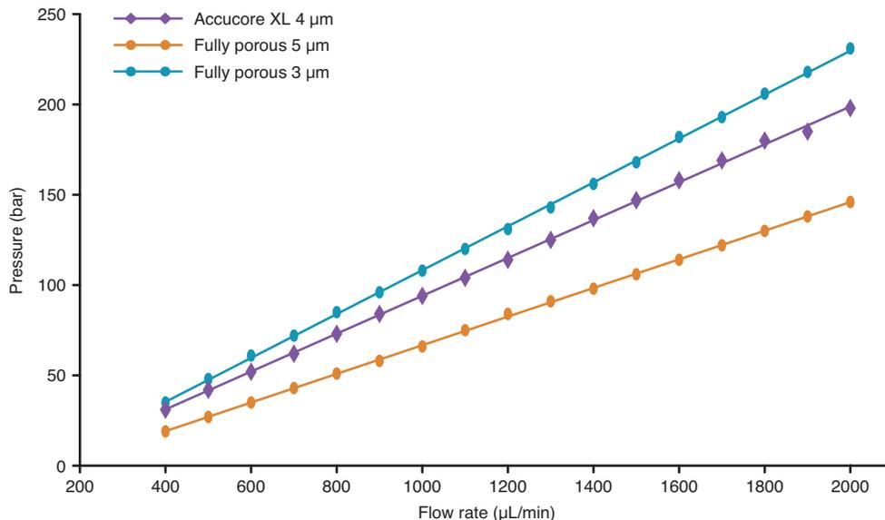
Figure 1: Comparison of column pressure for Accucore XL 4  $\mu\text{m}$  HPLC column and fully porous 5  $\mu\text{m}$  and 3  $\mu\text{m}$  columns. All columns: 150 x 4.6 mm; test conditions: mobile water / acetonitrile (50:50 v/v); column temperature: 30 °C.
