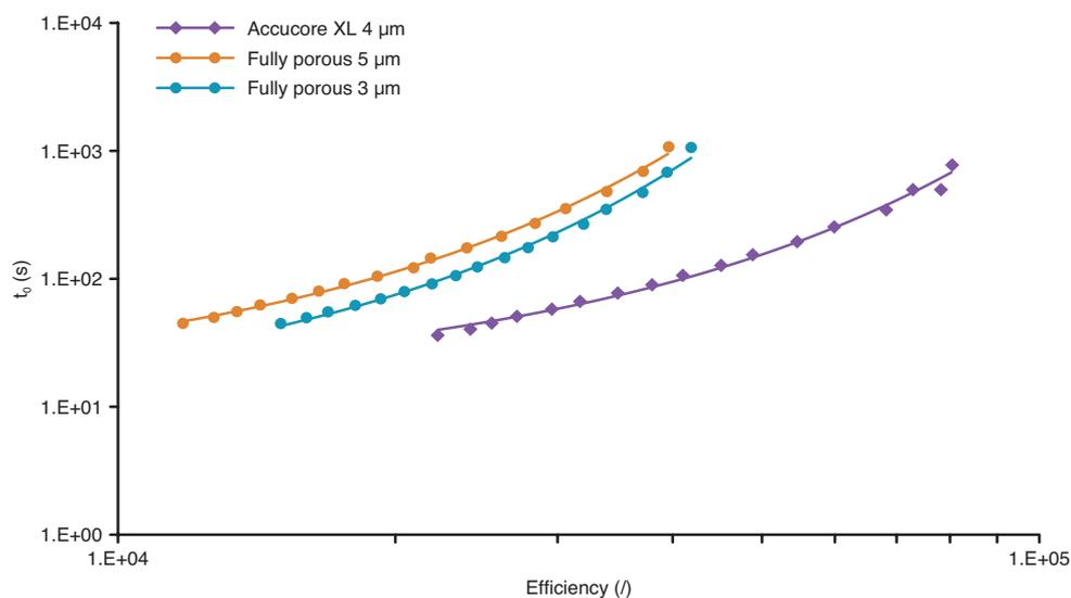
Figure 3: Performance comparison of Accucore XL 4  $\mu\text{m}$  HPLC column and fully porous 5  $\mu\text{m}$  and 3  $\mu\text{m}$  columns using kinetic plots: efficiency per unit time. All columns: 150 x 4.6 mm; test conditions: water / acetonitrile (50:50 v/v); column temperature: 30  $^{\circ}\text{C}$ ; test probes: o-xylene and theophylline ( $t_0$  marker).
