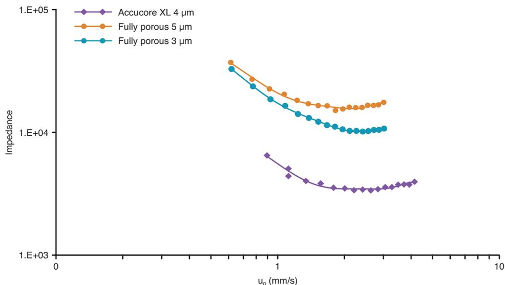
Figure 4: Performance comparison of Accucore XL 4  $\mu\text{m}$  HPLC column and fully porous 5  $\mu\text{m}$  and 3  $\mu\text{m}$  columns using kinetic plots: column impedance (E) relative to linear velocity (u). All columns: 150 x 4.6 mm; test conditions: water / acetonitrile (50:50 v/v); column temperature: 30  $^{\circ}\text{C}$ ; test probes: o-xylene and theophylline ( $t_0$  marker)
