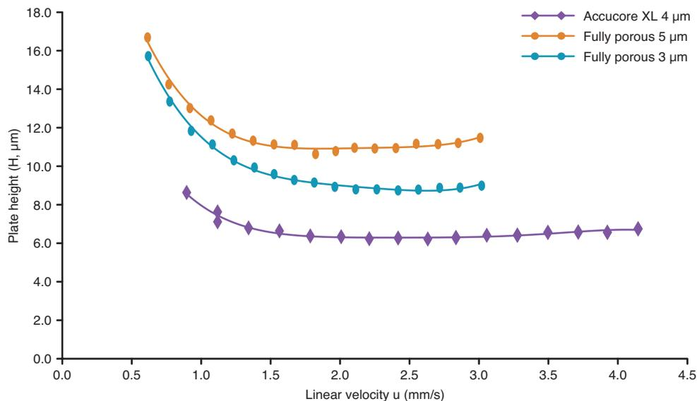
Figure 2: Efficiency comparison using van Deemter plots for Accucore XL 4  $\mu\text{m}$  HPLC column and fully porous 5  $\mu\text{m}$  and 3  $\mu\text{m}$  columns. All columns: 150 x 4.6 mm; test conditions: water / acetonitrile (50:50 v/v); column temperature: 30  $^{\circ}\text{C}$ ; test probes: o-xylene and theophylline ( $t_0$  marker).
