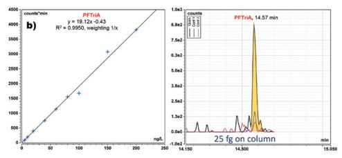
The LLOQs for all 24 PFAS analyzed in this method, based on accuracy and RSD  $\leq$ 20%, demonstrated the high sensitivity achieved with the TSQ Altis mass spectrometer for the quantitation of PFAS at very low levels (ppt range).
