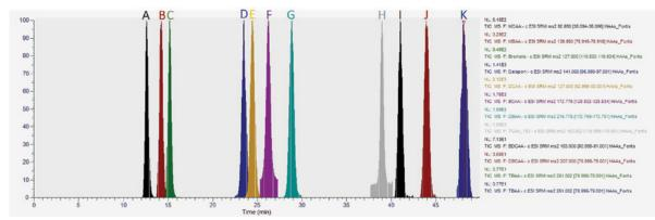
Ion chromatograms of HAAs: (A) MCAA, (B) MBAA, (C) Bromate, (D) Dalapon, (E) DCAA, (F) BCAA, (G) DBAA, (H) TCAA, (I) BDCAA, (J) DBCAA and (K) TBAA at 1  $\mu$ g/L.
