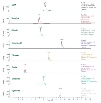
A good IC-MS/MS separation was achieved to resolve 16 analytes in different SRM channels. Fosetyl tends to degrade into phosphonic acid both in solution and in the IC-MS/MS via insource fragmentation. Phosphonic acid and fosetyl were fully separated on the Dionex IonPac AS19-4µm column with retention times of 8.92 min and 3.56 min, respectively.
