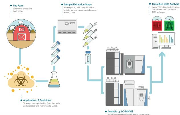
Perform targeted screening and/or quantitation using HRAM MS or QQQ MS, depending upon the experimental requirements
