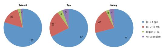
Relative percentages of different IDL values [ng/g] for the target compounds (328) in solvent, tea, and honey matrices. More than 85% of target compounds can be detected at  $\leq 10$  ng/g, and  $\sim 70\%$  of target compounds can be detected at  $\leq 1$  ng/g.
