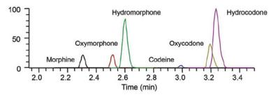
Chromatograms extracted from MS<sup>2</sup> spectra obtained from a confirmation PRM experiment for six opiates at their respective LOQs (2.5 ng/mL for codeine, oxycodone, and oxymorphone, and 5 ng/mL for hydrocodone, hydromorphone, and morphine) in hydrolyzed and diluted urine.
