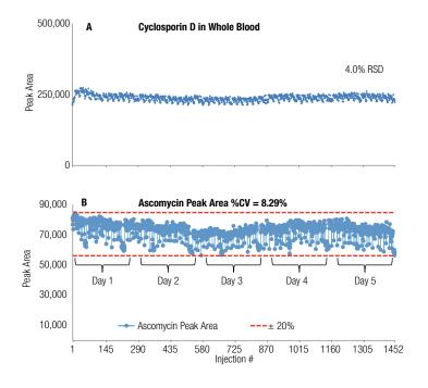
Peak areas for cyclosporin D and ascomycin, the two internal standards used in this study, showed precisions of 4% and 8%, respectively, over the five days and over 1500 injections.
