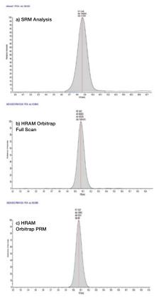
2.5 ppt standard of PFOA analyzed using the Q Exactive mass spectrometer and a triple quadrupole mass spectrometer under similar conditions. Excellent quantitative performance and sensitivity was obtained using the Q Exactive mass spectrometer in both full scan and PRM modes. The results obtained were equal to or better than the published LCMRLs using triple quadrupole SRM methods.
