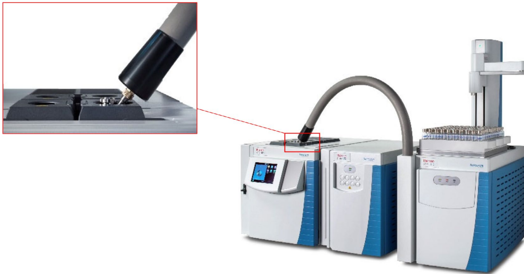
Figure 1. TRACE 1310 TOGA Analyzer connected to the TriPlus 500 HS. The HS transfer line connection to the GC inlet allows manual injection with a gas-tight syringe.
