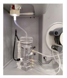
Figure 1. iCAP PRO XP ICP-OES or iCAP PRO XPS ICP-OES coupled with an integrated hydride generation kit
