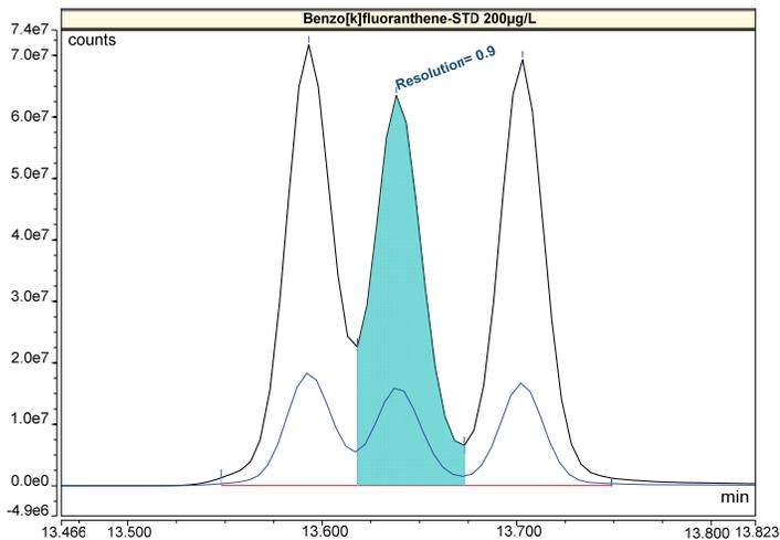
Figure 3. Separation of benzo[b] + benzo[k] + benzo[j]fluoranthene at 200 µg/L
