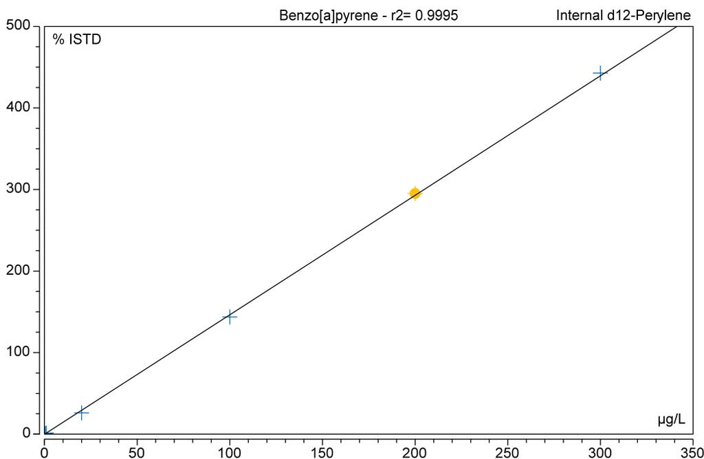
Figure 4. Calibration curve for benzo[a]pyrene. Six levels were used (0.4, 1, 20, 100, 200, 300 µg/L)
