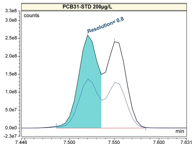
Figure 1. Separation of PCB 31 and PCB 28 at 200  $\mu$ g/L
