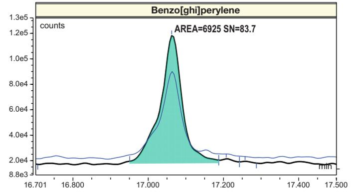
Figure 5. Overlaid SRM (quantifier ion in green, and qualifier ions in blue line) at 0.4 µg/L for a subset of analytes
