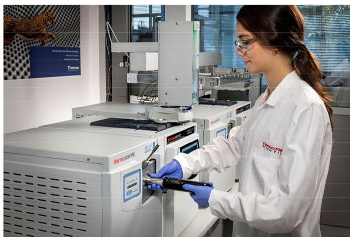
Figure 4. VPI being removed from the ISQ 7610 MS
