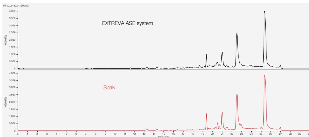
Figure 8. Chromatogram comparison of hexane extraction by the EXTREVA ASE system and 10 h SLE
