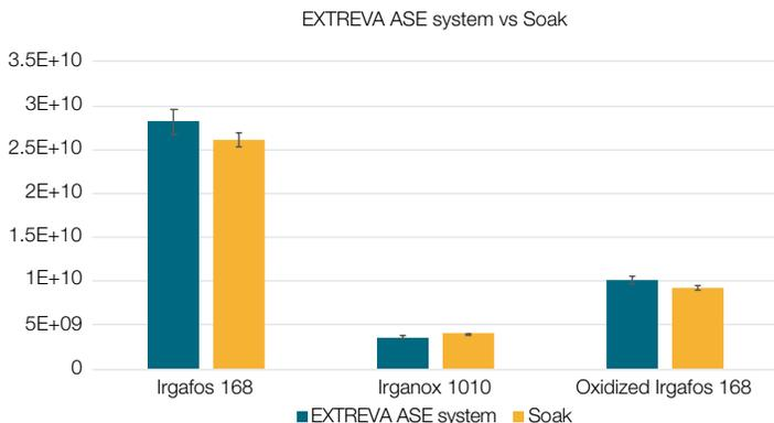
Figure 9. Comparison of hexane extraction by the EXTREVA ASE system and 10 h SLE
