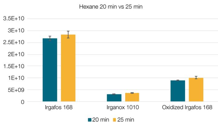
**Figure 7. Extraction of three additives using hexane with two different extraction times**
