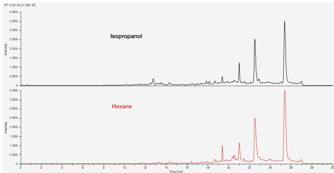
Figure 4. Total ion chromatogram of inhaler isopropanol and hexane extracts
