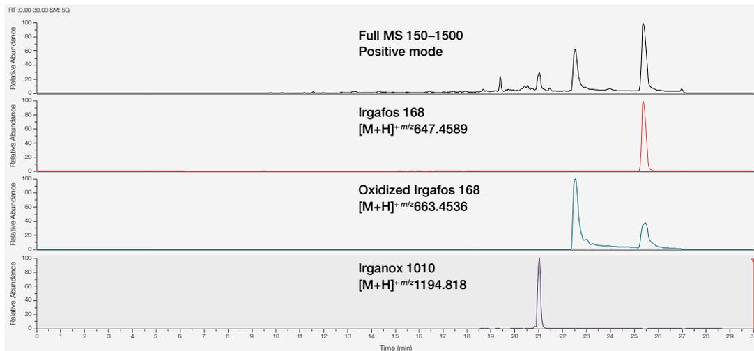
Figure 3. Total ion chromatogram (positive mode) of the inhaler hexane extract and extracted ion chromatograms of the three identified major compounds in the extract.
