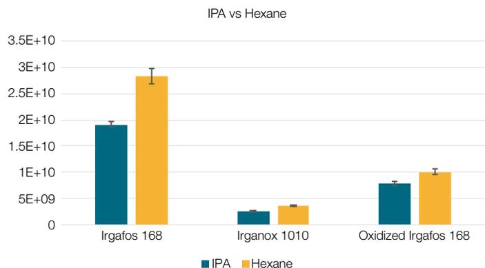
**Figure 5. Extraction of three additives using IPA vs hexane**
