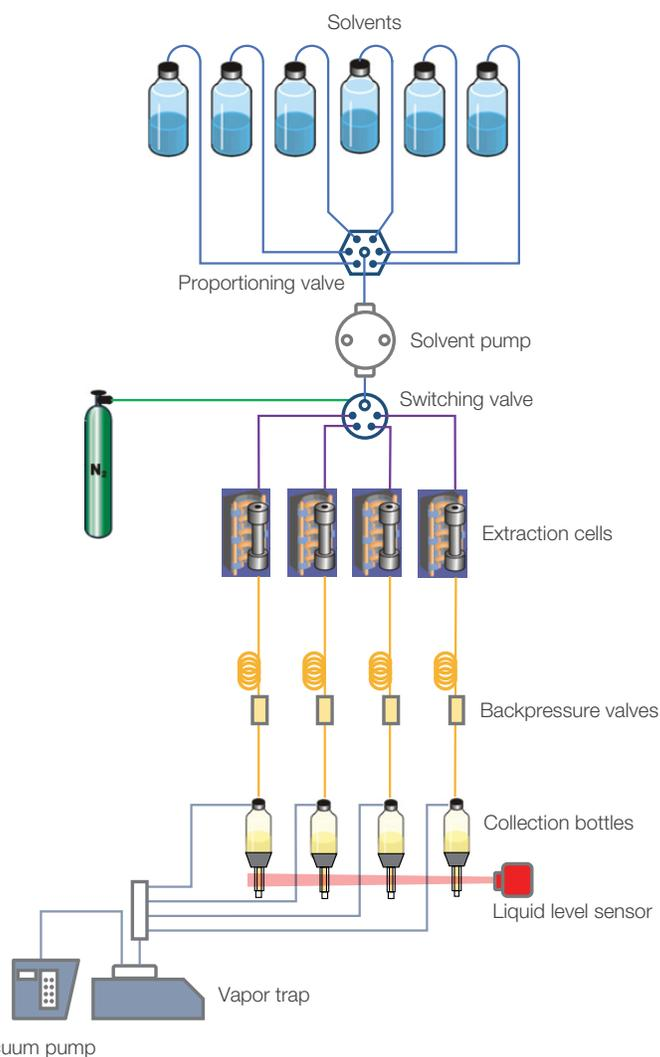
**Figure 2. Schematic diagram of the EXTREVA ASE Accelerated Solvent Extractor**
