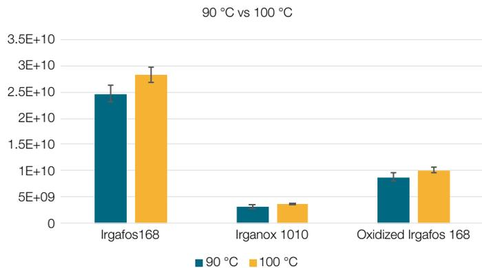
**Figure 6. Extraction of three additives using two different extraction temperatures**
