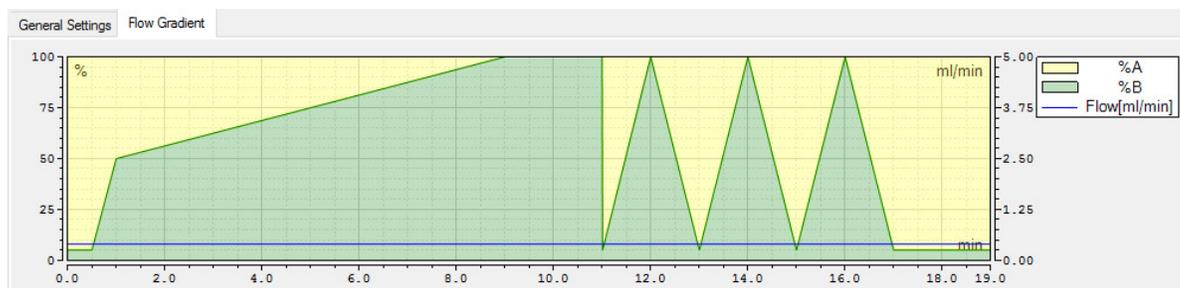
Figure 2. Gradient profile used for the analysis. A 'saw tooth' gradient at the end of run was found to reduce carryover of low-level PFAS from standards or matrix spikes.<sup>3</sup>
