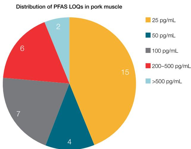
Figure 6. The limit of quantification (LOQ) distribution for the native PFAS are shown in the pie chart above. LOQ is defined here as MES % Average Recovery 60–130% and RSD < or = 25%.
