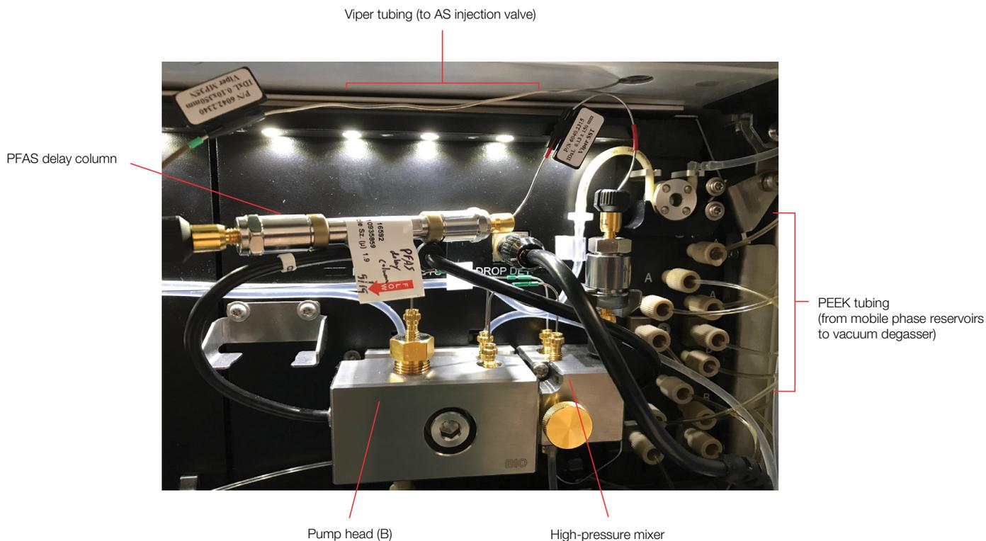
Figure 1. The Vanquish Flex UHPLC system shown here fitted with a PFAS Analysis Kit (P/N 80100-62142) that replaces wetted Teflon™ surfaces with comparable PEEK components and installing a PFAS trapping column.
