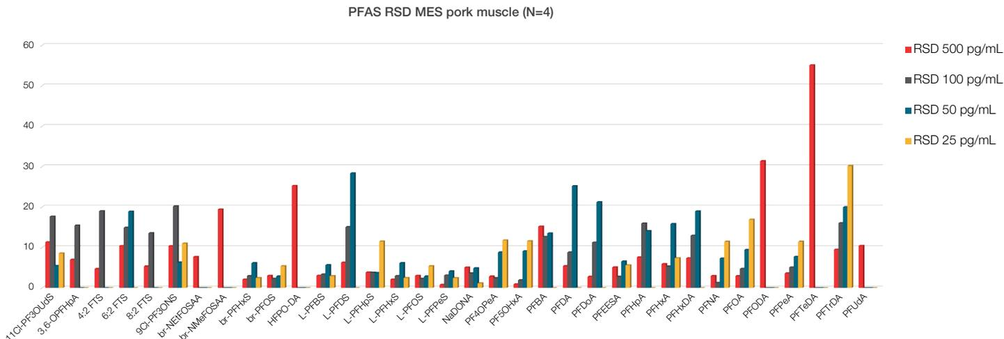
Figure 5. Average RSD of PFAS compounds based on four separate matrix extracted spikes of pork muscle meat at each concentration.
