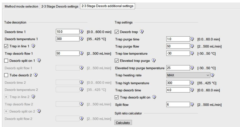
Figure 1. Chromeleon CDS browser showing the method editor wizard for the TD100-xr thermal desorption unit: (A) 2-3 Stage Desorb settings and (B) additional settings.
