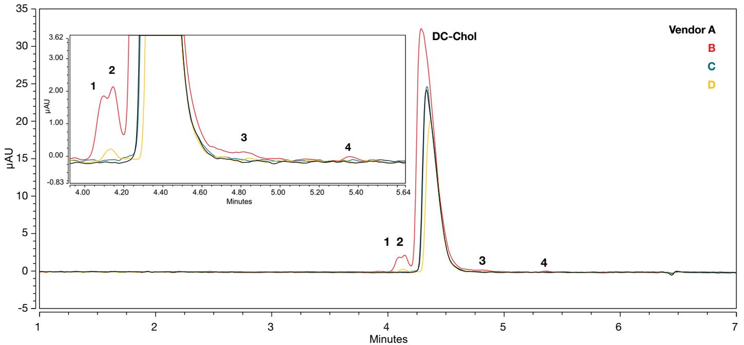
Figure 5. Overlay of the background-subtracted CAD traces for the DC-Chol raw material samples from vendors A–D, with inlaid detail of detected impurity peaks
