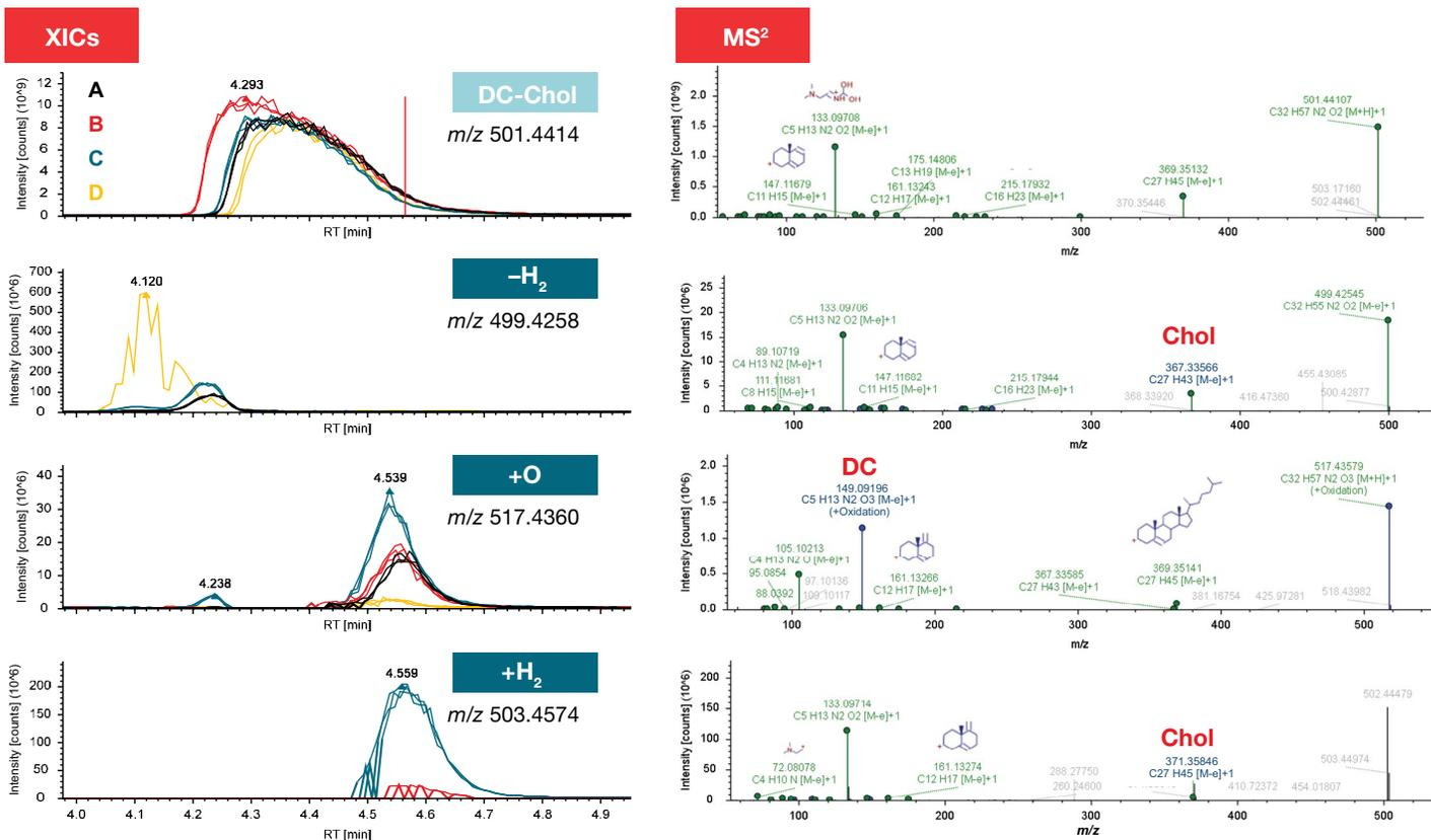
Figure 10. Detection of closely eluting trace impurities of DC-Chol from the MS data that were not detected in the CAD trace due to masking by the dominant main compound, and elucidation of the modification site based on the fragmentation spectra with transformation-shifted fragments highlighted in blue
