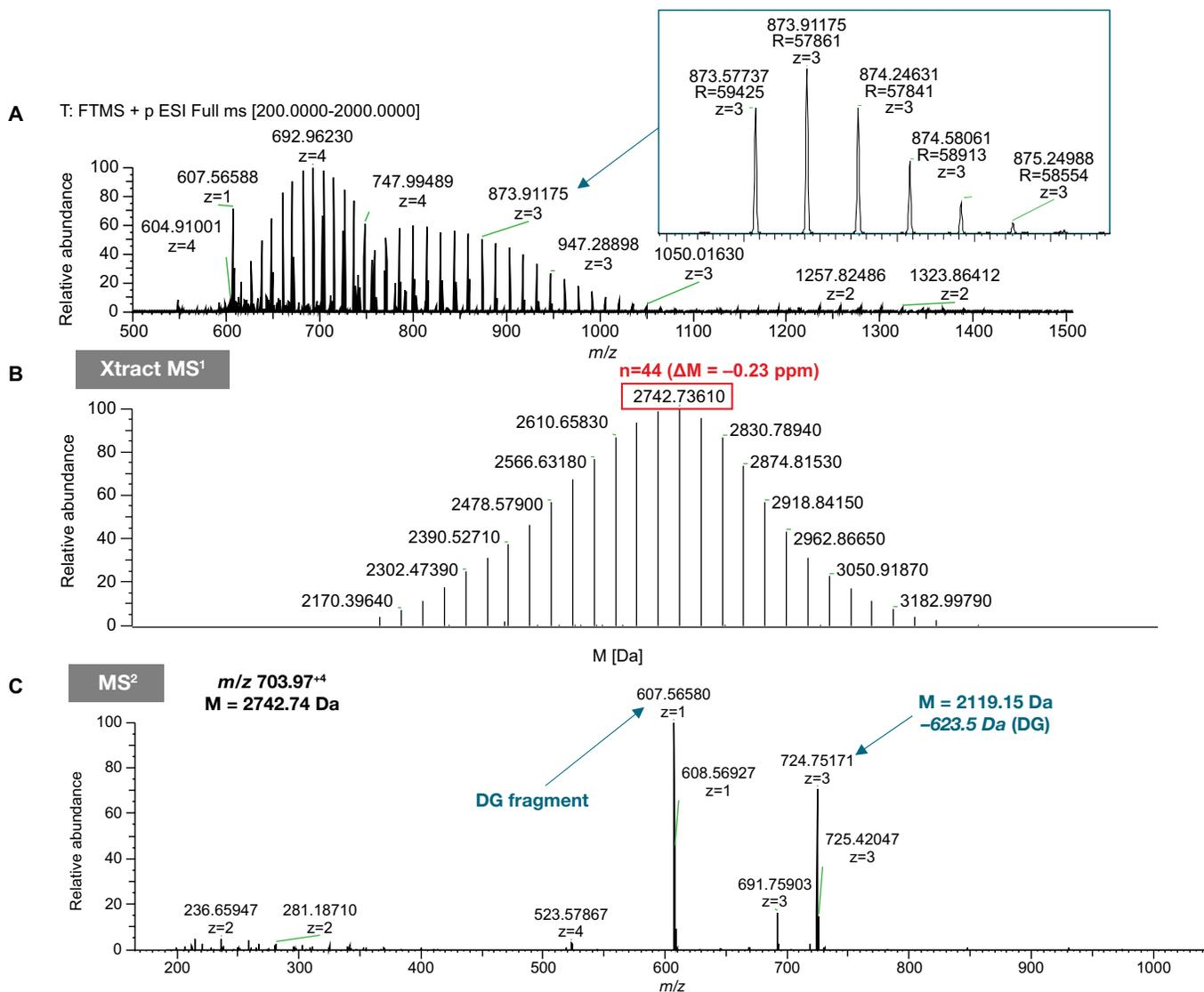
Figure 12. (A) Averaged mass spectrum of DSPE-mPEG from 4.8–5.4 min for vendor A, (B) deconvoluted mass spectrum showing the different polydispersity of the PEG chain lengths, and (C) evidence of the distearoyl glyceride in the fragmentation spectrum of the +4 ion of the most abundant species at MW 2742.74 Da
