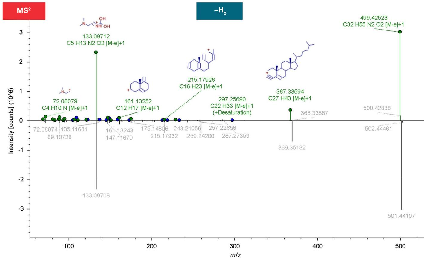
Figure 6. Correlation of CAD impurity peak 1 to the MS component for the desaturation transformation in Compound Discoverer 3.3 software, with the shifted fragment at *m/z* 367 compared to the parent compound allowing the localization of the additional double bond to the cholesterol moiety
