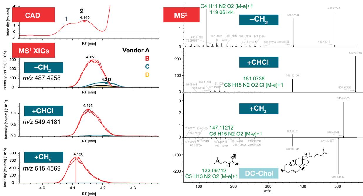
Figure 8. MS data correlated to impurity peak **2** in the CAD data reveals three co-eluting impurities with the MS<sup>2</sup> spectra indicating the respective transformations on the DC group
