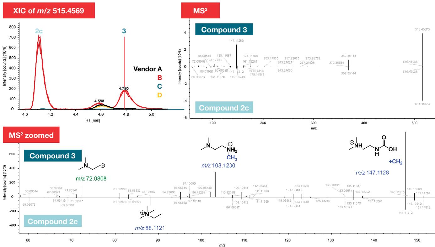
Figure 9. Comparison of isomeric impurities **3** and **2c** based on their XIC and fragmentation spectra, indicating their difference in methylation sites based on unique low *m/z* fragment ions
