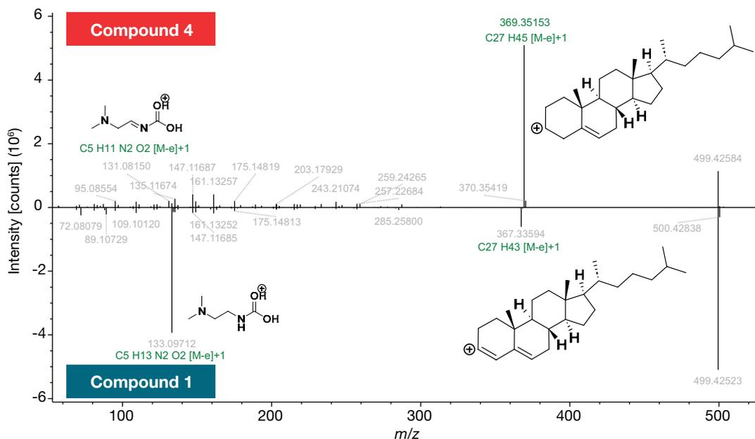
Figure 7. Differences in fragmentation spectra of isomeric impurities **1** and **4** allowing the determination of the respective transformation sites
