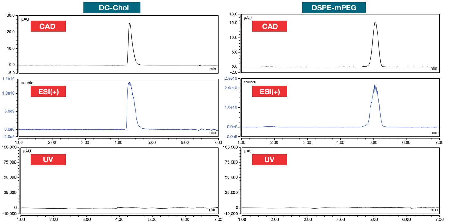
Figure 4. Representative LC/CAD/HRAM-MS chromatograms of DC-Chol and DSPE-mPEG from vendor A at 1 mg/mL concentration showing the correlation between CAD and MS peaks, and lack of signal in LC/UV analysis
