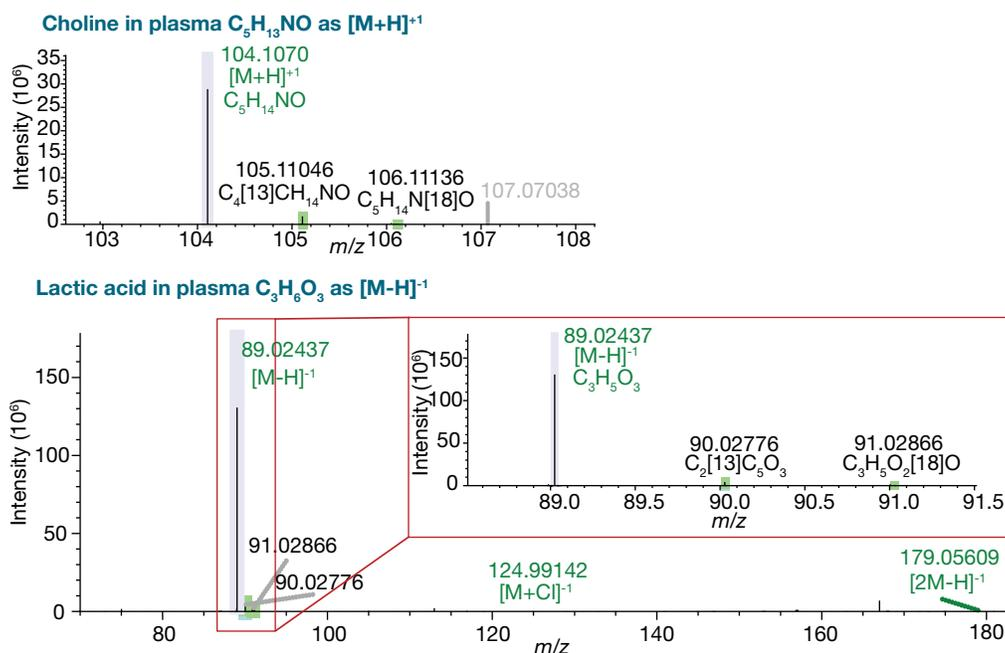
Figure 5. Two annotated compounds in plasma using the SQUAD analysis workflow on an Orbitrap Exploris MX mass detector, which provided high isotopic fidelity for compound identification. Lavender bars indicate the spectral peak in the isotope pattern with the highest intensity. Usually the most intense peak in an isotope pattern is the A0 peak for the monoisotopic ion. Green rectangles indicate matching centroids for isotopic ions.
