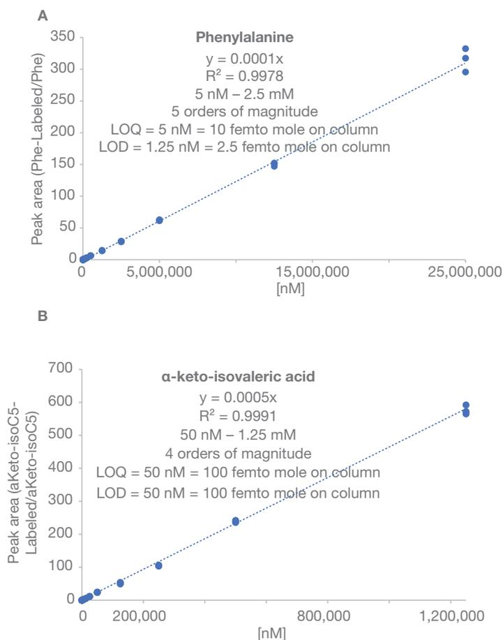
Figure 3. Absolute quantitation results for (A) phenylalanine and (B) alpha-keto-isovaleric acid spiked in NIST SRM 1950 plasma reference standard
