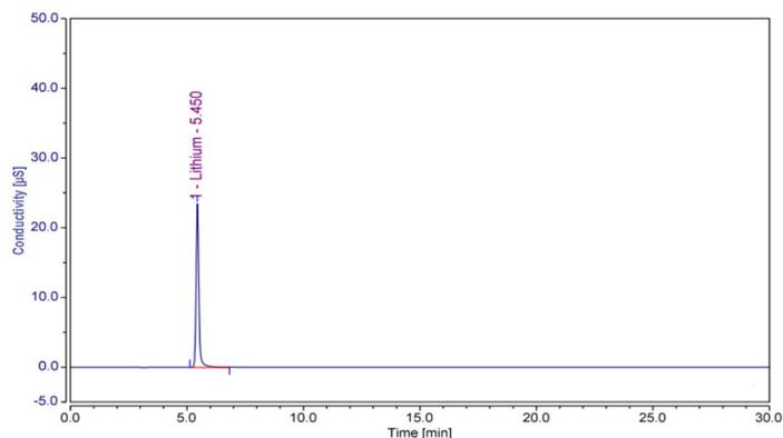
Figure 9. Chromatogram of lithium hydroxide monohydrate sample
