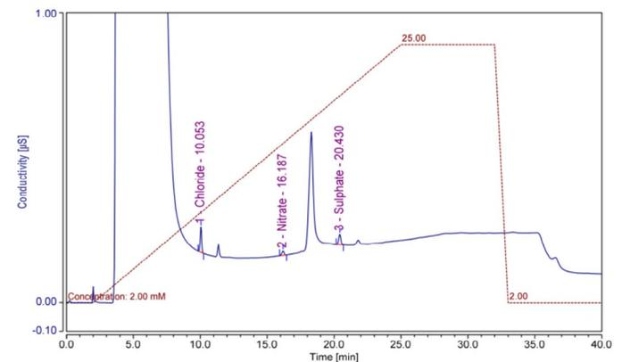
Figure 3. Chromatogram for lithium fluoride (B1)
