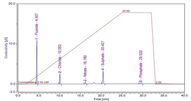
Figure 2. An example chromatogram for anionic impurities standard-3, showing excellent separation and resolution for all anions, with no interference from other compounds
