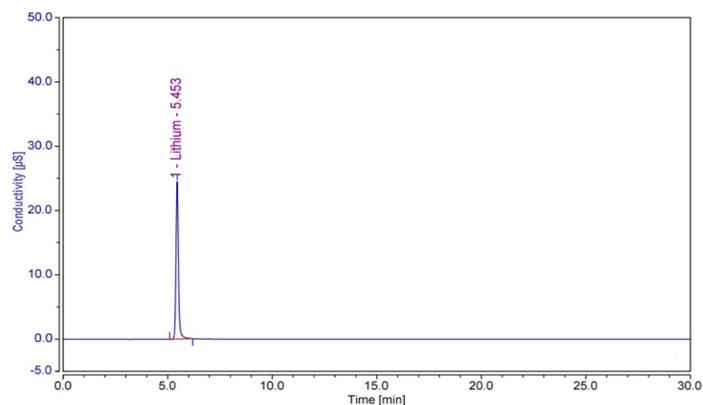
Figure 10. Chromatogram of lithium carbonate sample
