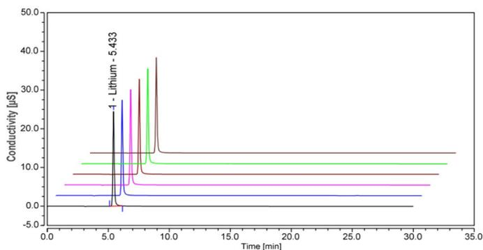
Figure 7. Chromatogram overlay (offset for conductivity and time, for clarity) for repeated injections of the 10 ppm lithium standard
