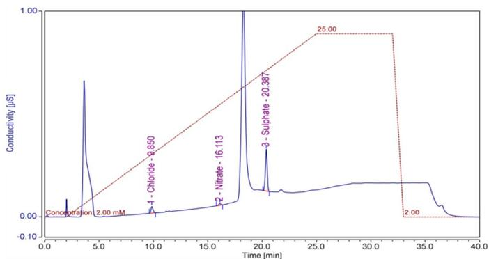
Figure 6. Chromatogram of lithium hydroxide monohydrate
