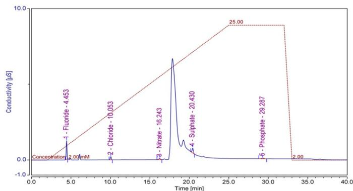
Figure 5. Chromatogram of lithium carbonate (B1)
