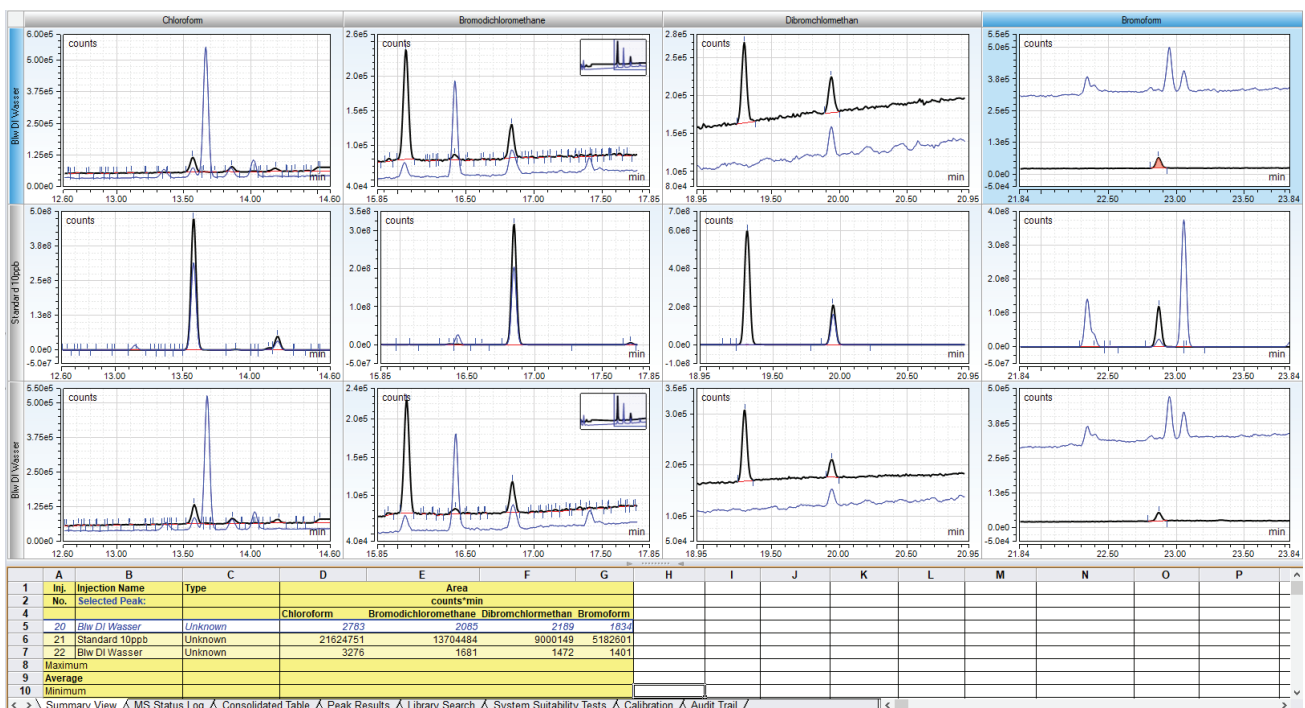
Figure 7. Carryover for all analytes is <0.027%. Top traces: clean DI-water before standard mix analysis. Middle traces: standard mixture at 10 µg/L. Bottom traces: clean DI-water after standard mix analysis.
