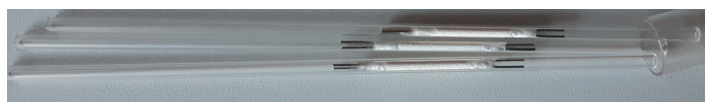
Figure 3. 2 mm ID packed deactivated glass liner for the iConnect PTV injector module
