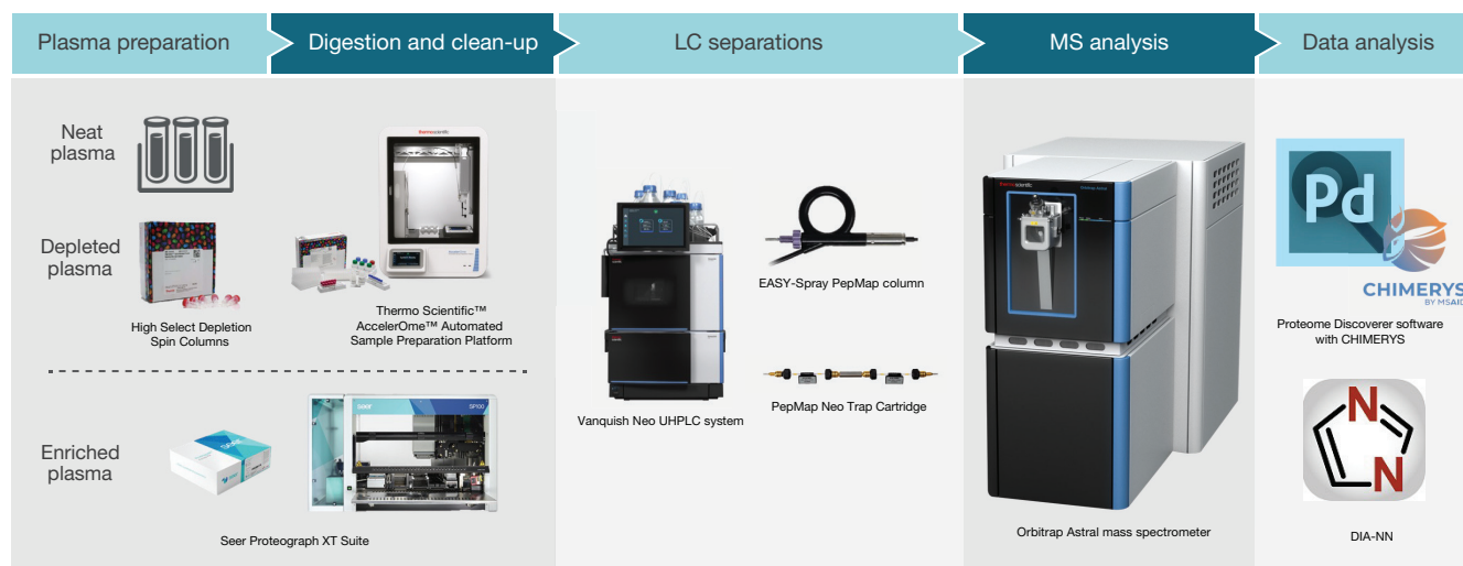
Figure 1. Schematic diagram of high-throughput plasma proteomics analysis powered by the Orbitrap Astral mass spectrometer.
