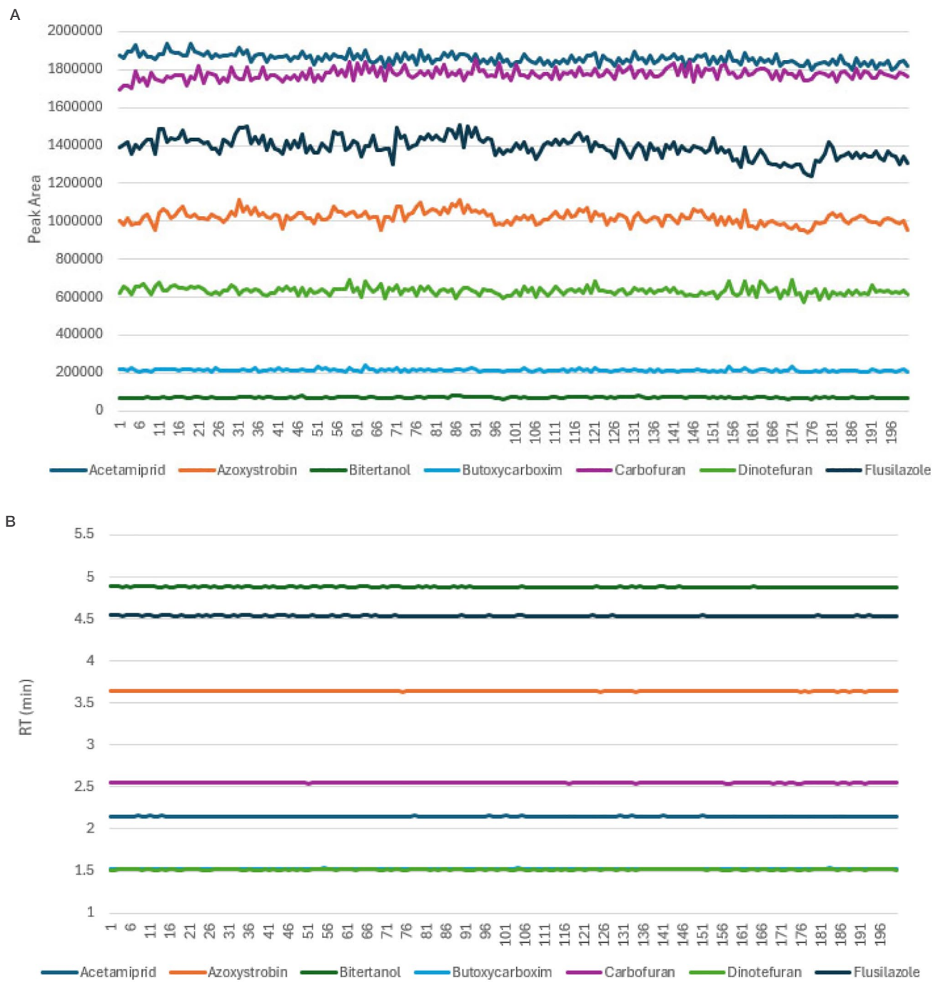
Figure 3. (A) Peak area stability for 200 injections of garlic extract spiked at 5 ppb for seven select pesticides chosen to cover a broad retention time in the method; (B) retention time stability for the same seven pesticides over 200 injections in the garlic extract
