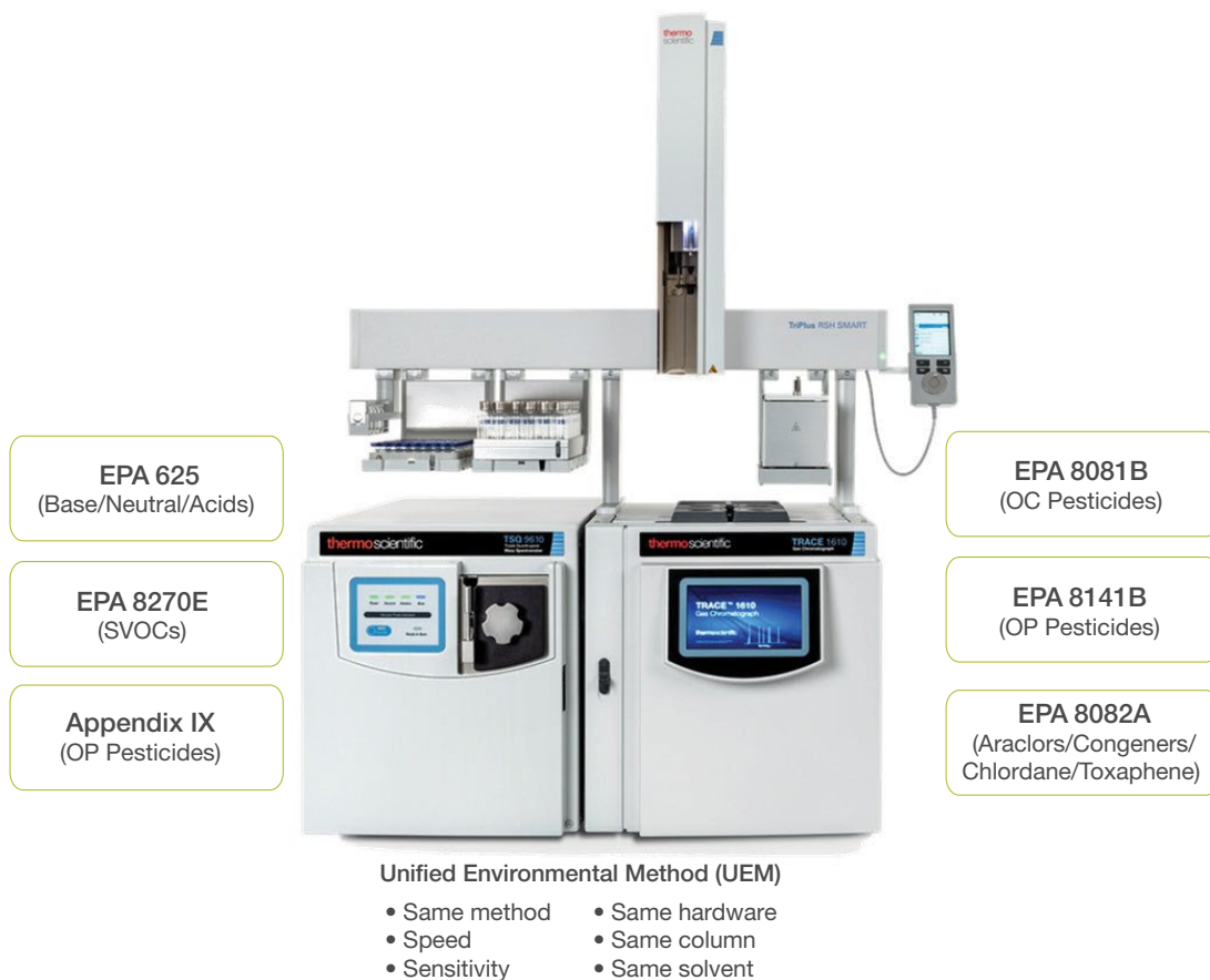
Figure 1. Unified environmental method schematic for analysis of multiple compound classes using a single analytical platform
