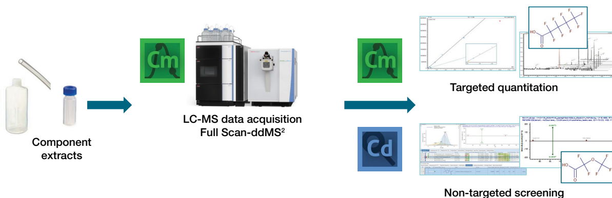
Figure 1. Overview of the LC-MS analytical strategy for detection of targeted and non-targeted PFAS as part of E&L analysis of pharmaceutical packaging and processing material extracts
