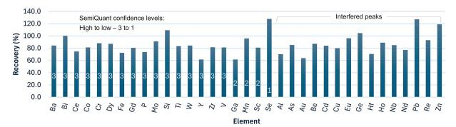
Figure 2. Spike recovery estimates, and respective confidence levels based on the number of reliable wavelengths used by the AI model, from semiquantitative analysis compared to expected spiked concentration of 0.1 mg·L<sup>-1</sup> in 10x diluted NASS-6
