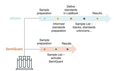
Figure 1. Workflows for eQuant and SemiQuant analysis using the iCAP PRO Series ICP-OES
