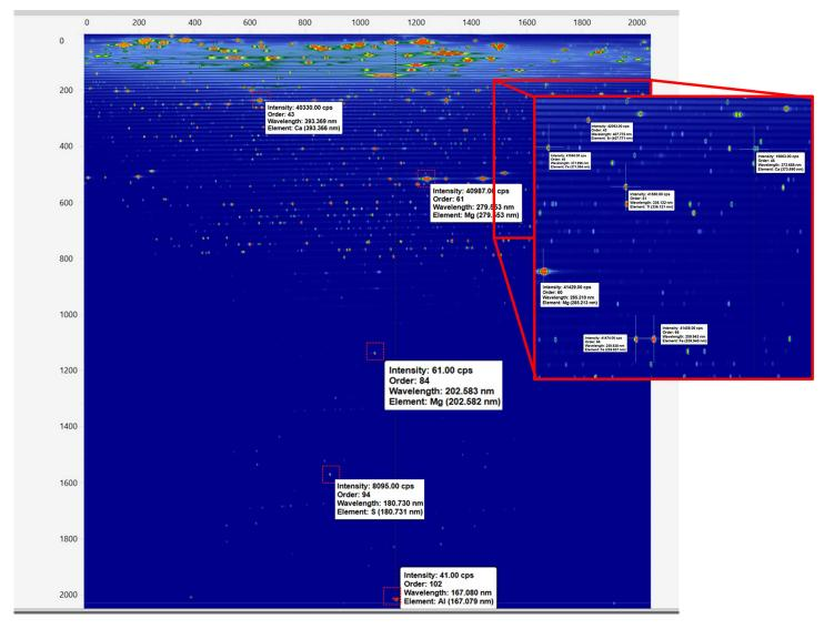
Figure 3. Full Frame image of an unknown sample from the iCAP PRO Series ICP-OES where the entire spectrum from 167 to 852 nm is captured simultaneously in a single exposure
