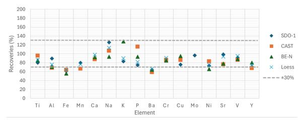
Figure 4. Accuracy of the semiquantitative measurements of geological samples in the present study compared to results obtained from XRF analysis. Low recoveries below 70% are linked to high concentrations of the respective matrix elements (e.g., up to 9% Fe in the rock samples).
