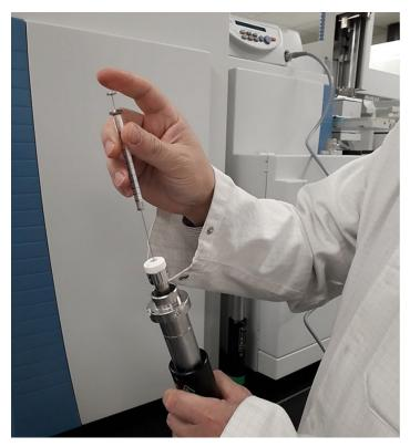
Figure 1. DIP sample loading procedure
