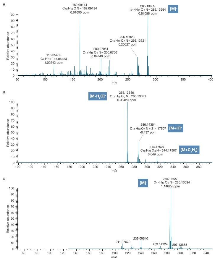
Figure 5. Confirmation of morphine-based mass accuracy measurements: (A) electron ionization mass spectrum, (B) positive chemical ionization mass spectrum, and (C) negative chemical ionization mass spectrum, annotated with mass (*m/z*), elemental composition, theoretical mass, and delta (ppm). Morphine molecular ion confirmed based on adducts formed ( $[M+H]^+$ ,  $[M+C_2H_2]^+$ ,  $[M]^-$ ) as well as excellent mass accuracy.
