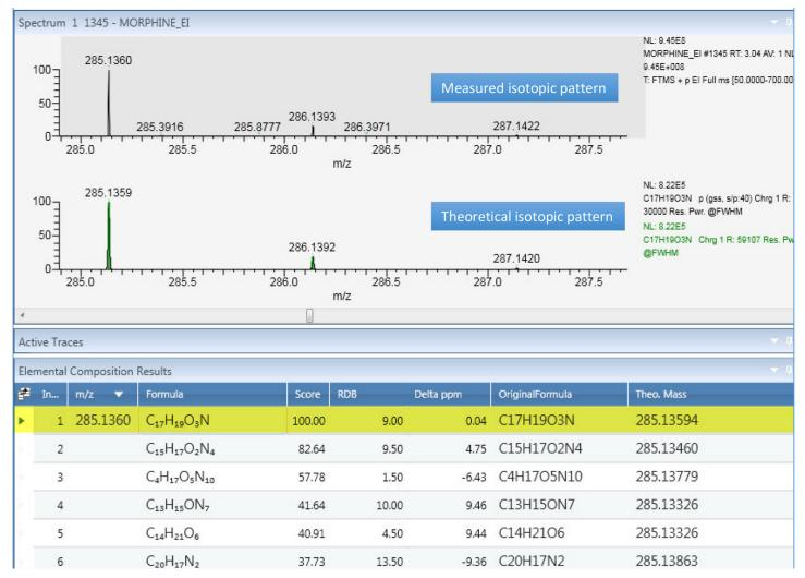
Figure 4. Elemental composition and isotopic pattern comparison for morphine indicating clearly  $C_{17}H_{19}O_3N$  as the most likely elemental composition with a mass accuracy of 0.04 ppm and an isotopic pattern score of 100% (direct match between measured versus theoretical isotopic match)
