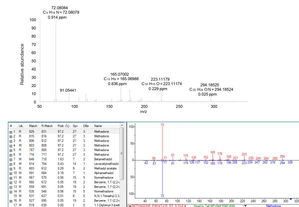
Figure 3. El mass spectra, corresponding accurate masses (ppm) and elemental composition. NIST library spectral match showing methadone (A) and morphine (B) as top hits with SI scores >830. Data acquired in El at 60,000 resolution (FWHM, at m/z 200).
