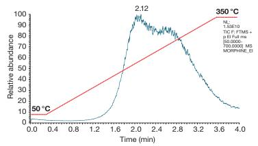
Figure 2. TIC of morphine analyzed using DIP-Orbitrap MS. The red dotted line represents the DIP probe programmed temperature rate. The components of the sample loaded are separated according to their boiling points up to highest masses selected in the full scan acquisition method. Data was acquired in full scan using El and 60,000 resolution.
